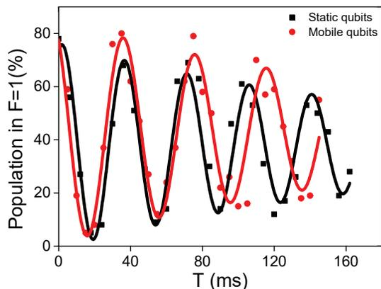
Figure 5. (Color online) Measured Ramsey signals for single static qubits (black square) and single mobile qubits (red dots) at  $B=3.115$  G. Every point is an average over 100 experimental runs. The solid curves are fits to the damped sinusoidal function. The fitted values of coherence times  $\tau$  of static qubits and mobile qubits are  $206 \pm 69$  ms and  $205 \pm 74$  ms respectively.
