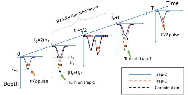
Figure 4. (Color online) Schematic illustration of the transfer process of a mobile qubit. An atom in a superposition state (the qubit) is initially confined in the static ODT (trap-2). It is then overlapped with the mobile ODT (trap-1). The qubit is extracted out by the mobile ODT and becomes a mobile qubit. The mobile qubit travels for time interval  $t$ , and then it is returned to the static ODT.
