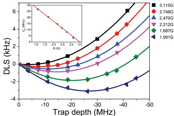
Figure 2. (Color online) DLS in the presence of hyperpolarizability. DLS of a qubit in the circularly polarized trap-2 is measured as a function of trap depths at various magnetic field strengths. The solid curves are fits to the Eq.(1). The inset plots the minima  $U_M$  in the DLS curves as a function of magnetic field  $B$ . The light intensity of each minimum is chosen as the magic intensity at that B-field value.
