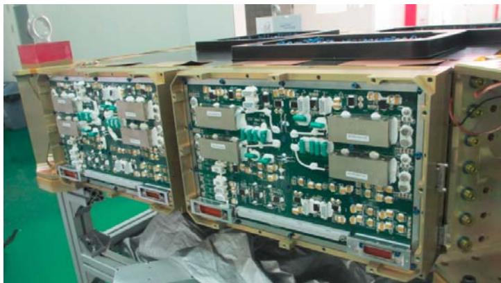
Fig. 5. Side View of the +X TRBs mounted on the framework of STK
