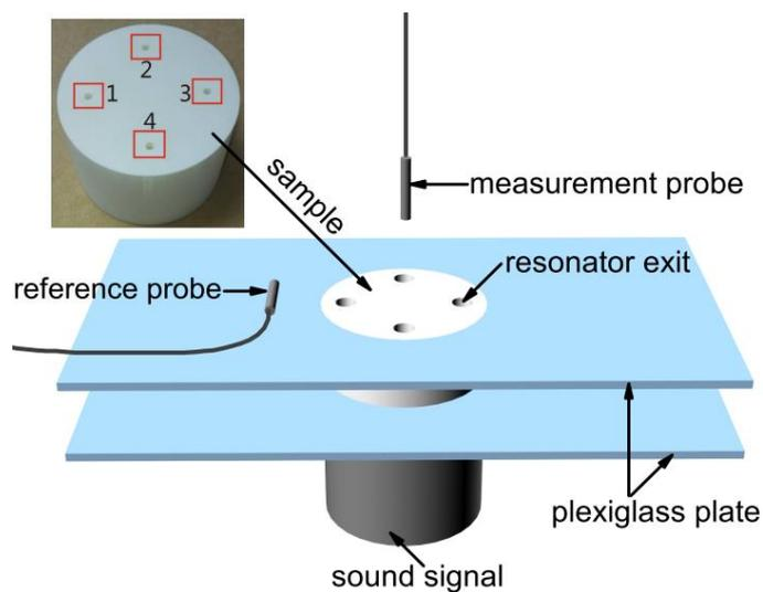
FIG. 3. Experimental setup for generating a sound vortex. The exits of the other resonators will be shielded if the sound response of a single resonator is measured.
