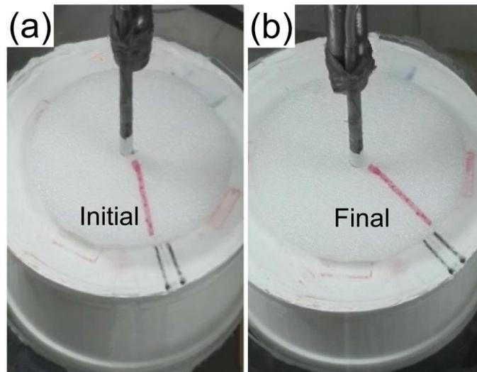
FIG 5. The torque effect exerted by the vortex beam on an absorbing foam disk that is suspended by a fine thread (not captured well by this top view), where (a) and (b) represent the initial and final states, respectively. Guiding lines are marked for a better observation of the disk rotation.
