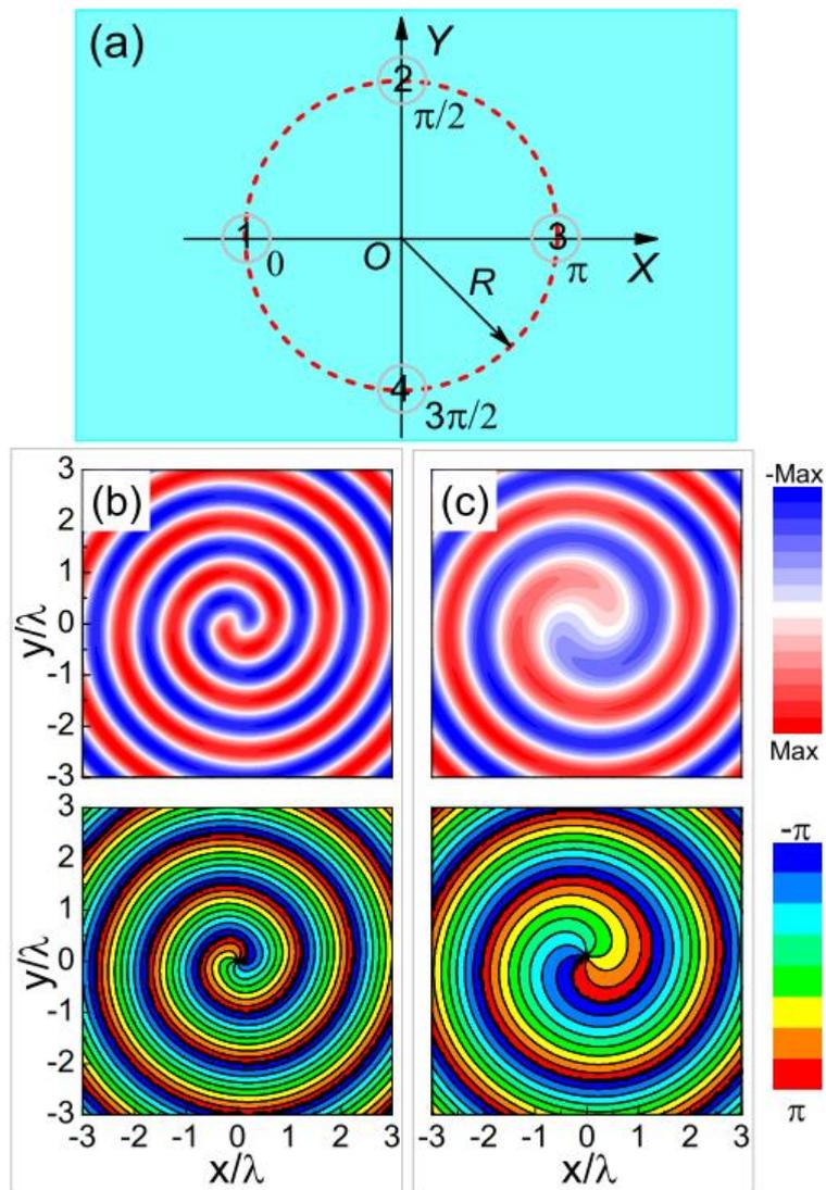
FIG. 1. Vortex design based on the Huygens-Fresnel principle. (a) Spatial distribution of four point sources with constant amplitudes and gradually varied phases. (b) The instant pressure profile (upper panel) and the corresponding phase pattern (bottom panel) superposed from the four point sources, evaluated for the plane  $z = 0.2\lambda$ . (c) The same as (b), but for the plane  $z = 2\lambda$ .
