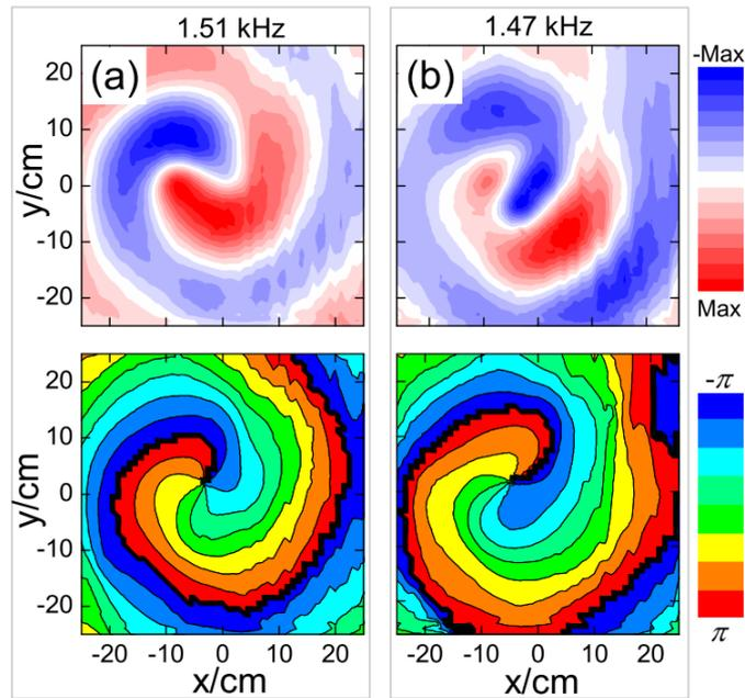
FIG 4. Instant pressure profiles (top panel) and phase patterns (bottom panel) scanned experimentally on the  $z = 4.0$  cm plane, with (a) for 1.51 kHz and (b) for 1.47 kHz.
