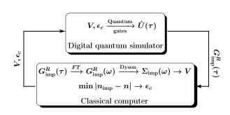
**Figure 2 Non-linear hybrid quantum-classical scheme.** A digital quantum simulator works in conjunction with a classical feedback loop to perform a proof-of-principle demonstration of a two-site DMFT calculation.
