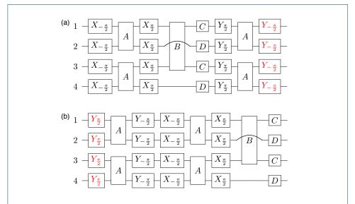
**Figure 4 Reordering of quantum gates.** The ordering of gates shown for (a) an odd Trotter step and (b) an even Trotter step in the CZ method. The gates depicted in red can be omitted as they cancel out during a sequence of time steps.
