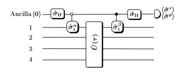
Figure 10 Quantum network to measure the  $\langle GS|\hat{U}^{\dagger}(\tau)\hat{\sigma}_{1}^{\alpha}\hat{U}(\tau)\hat{\sigma}_{1}^{\beta}|GS\rangle$  contribution to the Green function  $G^{R}_{\mathrm{imp}}(\tau)$ . The time-evolution operator  $\hat{U}(\tau)$  is composed of a set of quantum gates according to the main text.
