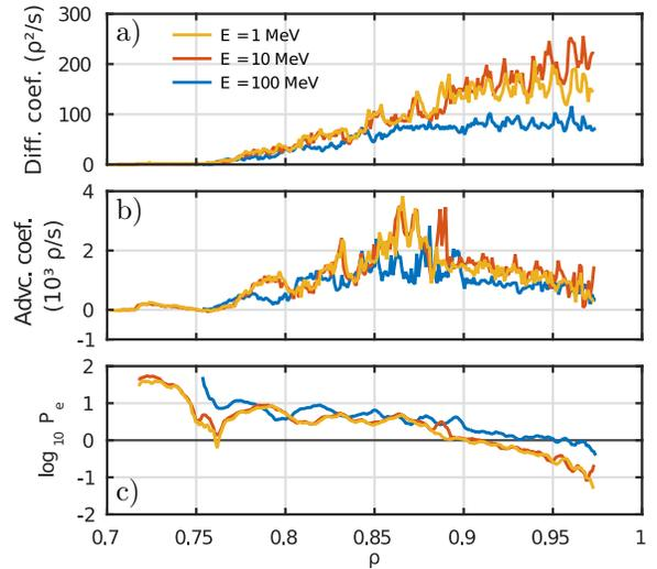
**Figure 9.** The transport coefficients and Péclet number from Fig. 4 shifted radially outwards in  $\rho$  by a  $\Delta\rho = [\text{orbit width}]/\sqrt{2}$ , which is the RMS value of the particle excursion from its initial  $\rho$  surface over the course of its poloidal turn.
