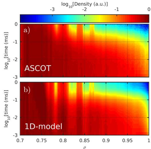
**Figure 6.** The particle density evolution in ASCOT (a) and 1D-model (b) for electron population with ( $E = 1$  MeV,  $\xi = 0.9$ ) in a magnetic field shown in Fig. 1. The full 3D simulation with ASCOT required approximately 600 cpu-hours while only a few minutes were needed with the 1D-model.
