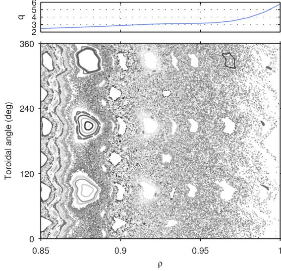
**Figure B1.** The magnetic field structure corresponding to ITER  $I_p = 15$  MA baseline scenario involving perturbations from ferritic inserts, test blanket modules, and RMP coils. The RMP coil current configuration is: mode  $n = 3$  and amplitude 45 kAt maximum current. Here  $J = \partial R / \partial \rho \approx 2.2$  m.
