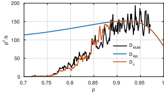
**Figure 5.** Numerical diffusion coefficient  $D_{\text{NUM}}$  for ( $E = 1$  MeV,  $\xi = 0.9$ ) electrons compared to the Rechester Rosenbluth result  $D_{\text{RR}}$ , Eq. (2), and to the form  $D_c$ , Eq. (20). The coefficients are for the field in Fig. 1. Here, the constant  $C$  has a value of  $C = 0.025$  for both  $D_{\text{RR}}$  and  $D_c$ . Note that  $D_{\text{RR}}$  and  $D_c$  overlap when  $\rho > 0.88$ .
