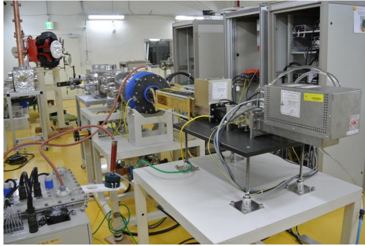
Fig. 9. Microwave ion source test stand
