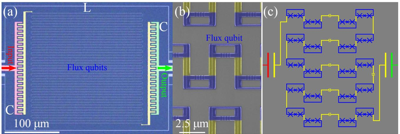
FIG. 1. Our device is composed of 4300 superconducting flux qubits embedded in an LC resonator. These flux qubits are coupled with the resonator via mutual inductance. We show in (a) an optical microscope image, (b) a scanning electron micrograph (in false colors), and (c) a schematic view of our device. Spectroscopy is performed on this device by measuring the photons transmitted from the resonator.
