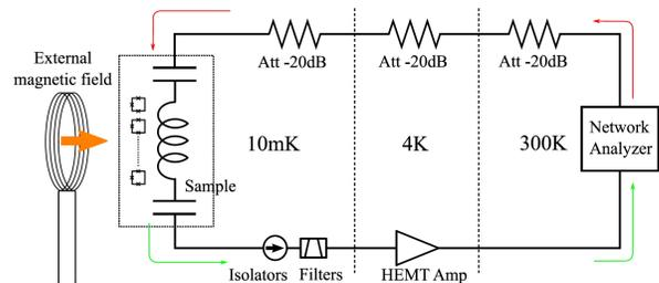
FIG. 3. Schematic of our experiment setup. Here, we measure the microwave transmission properties of the resonator with a network analyzer. The microwave resonator is inductively coupled with 4500 flux qubits.
