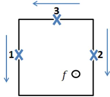
FIG. 4. Schematic of a superconducting flux qubit with three Josephson junctions. The area of one junction is designed to be  $\alpha$  times smaller than those of the other two junctions.
