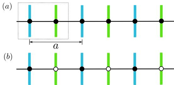
FIG. 1: Illustration of nonsymmorphic symmetries in one-dimensional lattices. (a) The nonsymmorphic symmetry is composed of a  $\pi$  rotation followed by a half translation  $a/2$ , where  $a$  is the lattice constant. (b) The nonsymmorphic *magnetic* symmetry is composed of the two operations of (a) followed by the exchange of black and white balls, which represents time-reversal symmetry.
