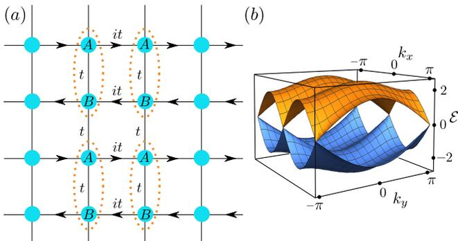
FIG. 4: (a) Illustration of the  $\pi$ -flux square lattice model. This model is invariant under the nonsymmorphic magnetic symmetry  $G(k_y)\hat{K}\hat{i}$ , namely a time-reversal symmetry followed by the nonsymmorphic symmetry  $G(k_y)$ . (b) Energy spectrum of the  $\pi$ -flux square lattice model.
