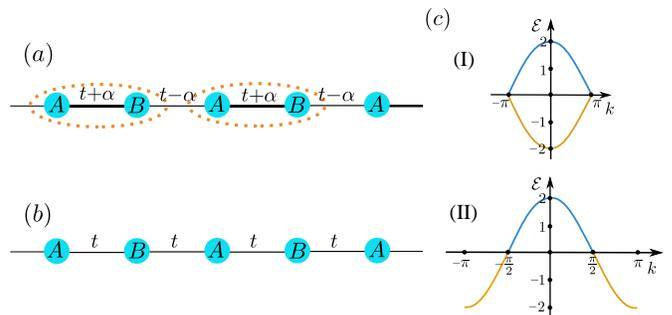
FIG. 3: Illustration of the SSH model. (a) For  $\alpha \neq 0$  the SSH model breaks the nonsymmorphic symmetry  $G(k)$ , Eq. (1). (b) At the critical point  $\alpha = 0$  the translation symmetry is promoted from  $2\mathbb{Z}$  to  $\mathbb{Z}$ , such that the nonsymmorphic symmetry  $G(k)$  is satisfied. (c) Energy spectrum at  $\alpha = 0$  in (I) the original BZ and (II) the unfolded BZ.
