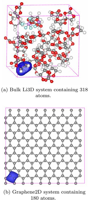
FIG. 5. Prototype 2D and 3D systems used for the computations in this work. Larger sized systems were obtained by periodic replication of these unit cells. Iso-surface of the first ALB from one of the DG elements of these systems is also shown.
