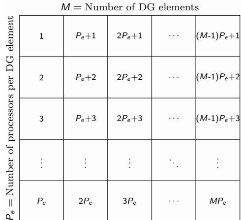
FIG. 2. Two-level parallelization scheme within DGDFE : The number of DG elements is  $M$  and each element has  $P_e$  processors dedicated to it, making the total number of processors  $P_{\text{tot}} = M \times P_e$ .
