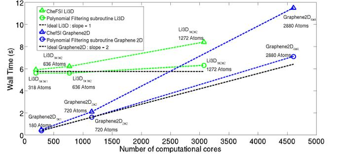
FIG. 8. Weak scaling performance of CheFSI in DGDFT. Performance of the filtering routine is also shown.
