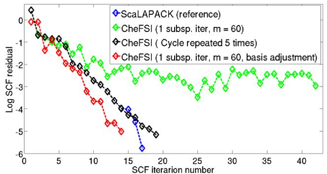
FIG. 3. SCF convergence of normalized electron density residual for different variants of CheFSI within DGDFT (naive implementation, multiple cycles, and eigenvector re-alignment to adjust for evolving basis set) for a simple system containing a few hydrogen atoms. Reference ScaLAPACK results are also presented.
