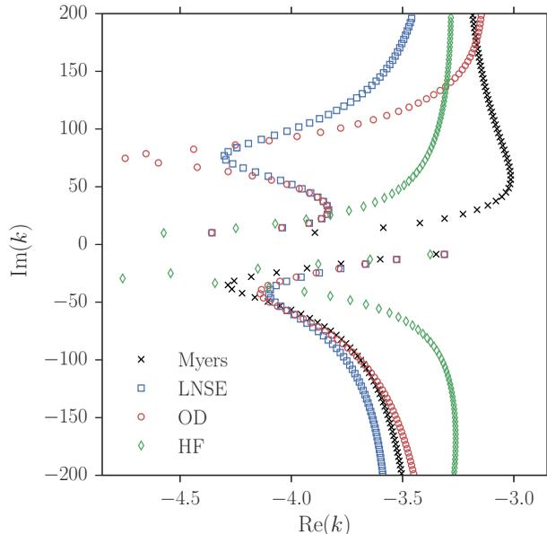
Figure 16. Cutoff modes in the  $k$ -plane of the Myers boundary condition, the LNSE numerics, the high frequency (HF) asymptotics (5.13) and the  $\mathcal{O}(\delta)$  (OD) asymptotics (5.2e) for  $\omega = 5$ ,  $m = 2$ ,  $\text{Re} = 1 \times 10^5$ ,  $\delta = 4 \times 10^{-3}$ . The boundary impedance  $Z$  is found using (2.10) with  $d = 0.08$ ,  $b = 6$  and  $R = 1.6$ . Base profiles as in (2.4b).
