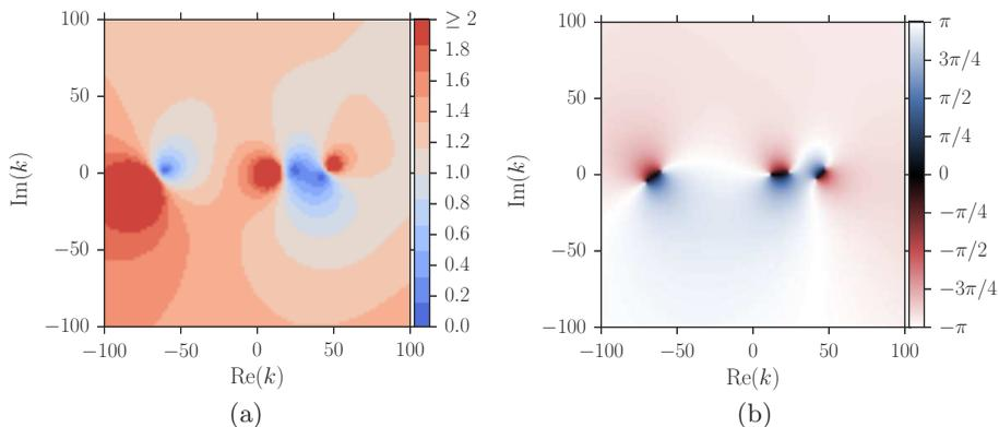
Figure 17. Contour plots in the  $k$ -plane of (a)  $|Z_{\text{eff}}/Z|$ , (b)  $\arg(Z_{\text{eff}}/Z)$  for the experimental setup of Jones *et al.* (2005), with  $f^* = 2500\text{Hz}$ ,  $Z = 0.93 - 1.43i$ ,  $M = 0.335$ . For a duct radius  $l^* = 1.5\text{m}$  and sound speed  $c_0^* = 340\text{ms}^{-1}$ , our dimensionless parameters are  $\omega = 69.3$ ,  $m = 0$ ,  $\text{Re} = 3.4 \times 10^7$ ,  $\delta = 9\%$ . Base profiles as in (6.3).
