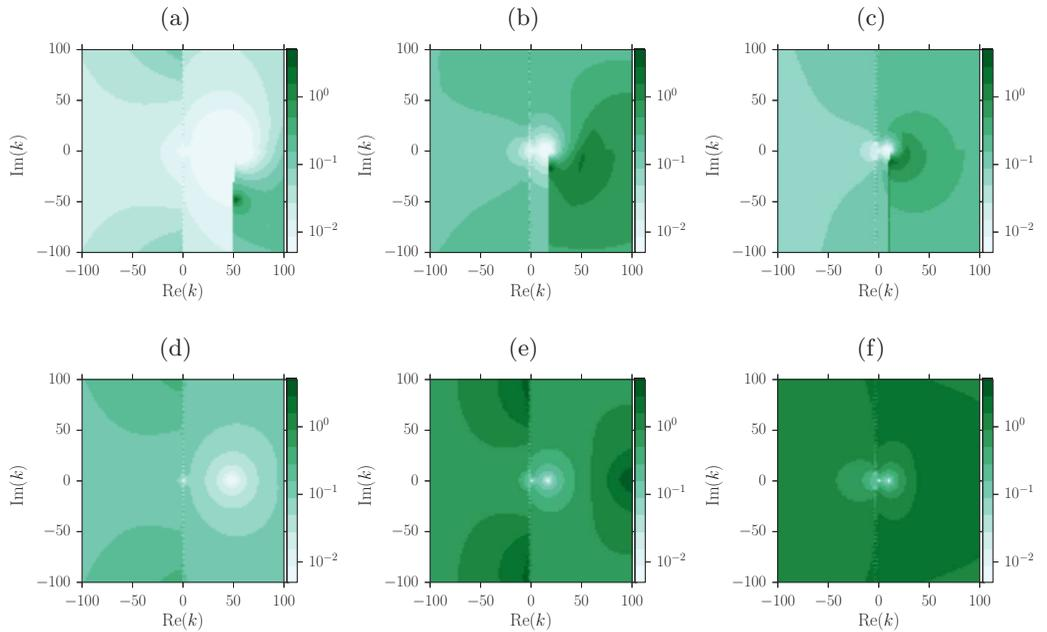
Figure 6. (a,b,c) viscous impedance error. (d,e,f) shear impedance error. (a,d)  $M = 0.1$ ; (b,e)  $M = 0.3$ ; (c,f)  $M = 0.5$ . Parameters are  $\omega = 5 + 0.05i$ ,  $m = 7$ ,  $\text{Re} = 5 \times 10^6$ ,  $\delta = 2 \times 10^{-3}$ . Base profiles as in (2.4b).
