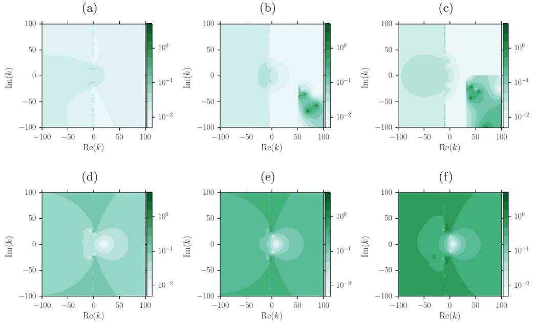
Figure 5. (a,b,c) viscous impedance error. (d,e,f) shear impedance error. (a,d)  $M = 0.1$ ; (b,e)  $M = 0.3$ ; (c,f)  $M = 0.5$ . Parameters are  $\omega = 15 + 0.15i$ ,  $m = 24$ ,  $\text{Re} = 1 \times 10^5$ ,  $\delta = 3 \times 10^{-2}$ . Base profiles as in (2.4b).
