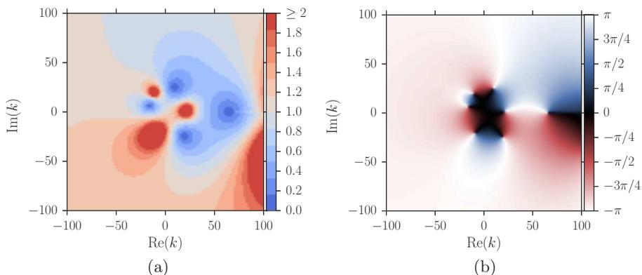
Figure 18. Contour plots in the  $k$ -plane of (a)  $|Z_{\text{eff}}/Z|$ , (b)  $\arg(Z_{\text{eff}}/Z)$  for the experimental setup of Marx *et al.* (2010), with  $f^* = 1200\text{Hz}$ ,  $Z = 0.25 - 0.39i$  and  $M = 0.32$ . For a duct radius  $l^* = 1\text{m}$  and sound speed  $c_0^* = 363\text{ms}^{-1}$ , dimensionless parameters are  $\omega = 20.8$ ,  $m = 0$ ,  $\text{Re} = 2.4 \times 10^7$ ,  $\delta = 5\%$ . Base profiles as in (6.3).
