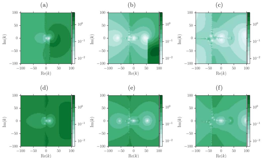
Figure 4. (a,b,c) viscous impedance error. (d,e,f) shear impedance error. (a,d)  $\omega = 7 + 0.07i$ ; (b,e)  $\omega = 28 + 0.28i$ ; (c,f)  $\omega = 56 + 0.56i$ . Parameters are  $m = 12$ ,  $M = 0.5$ ,  $\text{Re} = 1 \times 10^5$ ,  $\delta = 2 \times 10^{-3}$ . Base profiles as in (2.4b).
