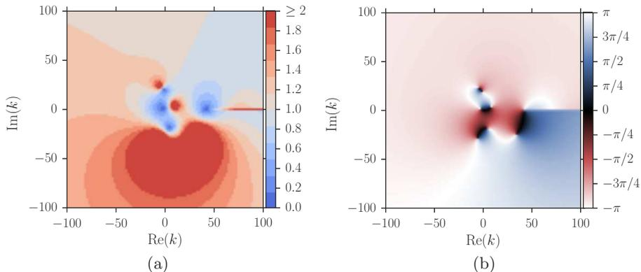
Figure 19. Contour plots in the  $k$ -plane of (a)  $|Z_{\text{eff}}/Z|$ , (b)  $\arg(Z_{\text{eff}}/Z)$  for the experimental setup of Jones *et al.* (2005), with  $f^* = 500\text{Hz}$ ,  $Z = 0.61 - 0.59i$  and  $M = 0.335$ . For a duct radius  $l^* = 1.5\text{m}$  and sound speed  $c_0^* = 340\text{ms}^{-1}$ , dimensionless parameters are  $\omega = 13.9$ ,  $m = 24$ ,  $\text{Re} = 3.4 \times 10^7$ ,  $\delta = 9\%$ . Base profiles as in (6.3).
