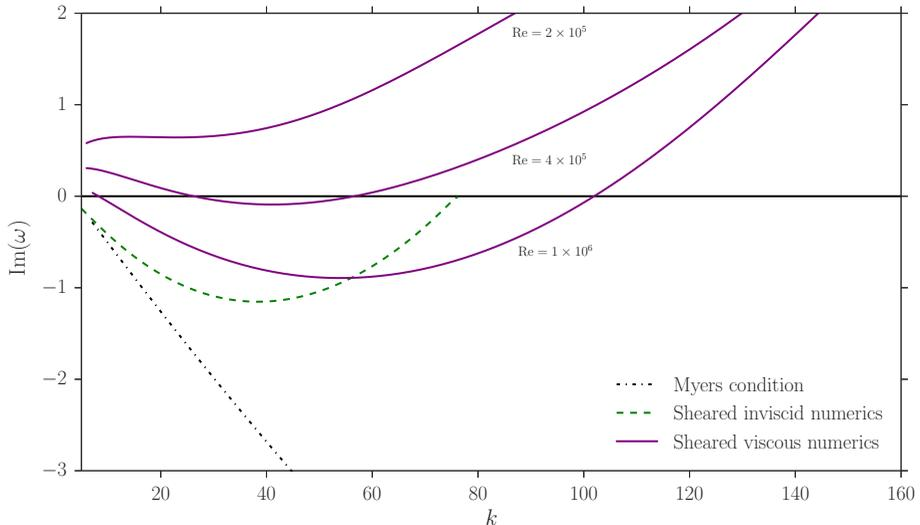
Figure 10. The decay rate  $\text{Im}(\omega)$  of the unstable mode is plotted as the real wavenumber  $k$  increases. The mode stabilises as  $\text{Re}$  is decreased past  $\text{Re} = 4 \times 10^5$ . Parameters are  $m = 0$ ,  $M = 0.5$ ,  $\delta = 5 \times 10^{-3}$ , with the mass–spring–damper liner model of (2.10), with  $R = 3$ ,  $d = 0.15$ ,  $b = 1.15$ . The hyperbolic base profiles (2.4b) are used.
