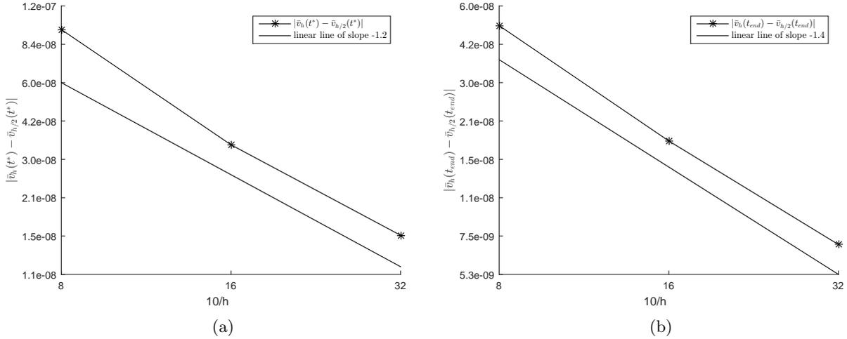
Figure 5.3: Void size difference between two consecutive discretization levels (a) at time  $t^*$  when the void is formed for the first time and (b) at time  $t_{\text{end}}$  when the mold is completely filled except the void.
