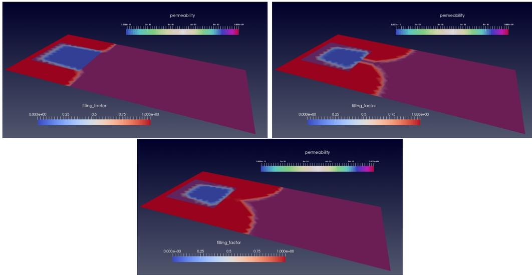
Figure 3.2: Void formation. The thickness of the material is 1cm, the inlet pressure  $p_I = 0.6\text{MPa}$ , the outlet pressure  $p_0 = 0.1\text{MPa}$ , and the porosity  $\varkappa = 0.7$ . The other parameters are given in Fig. 3.1.
