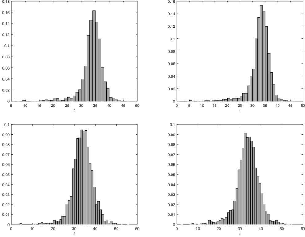
Figure 5.4: Sample densities for  $\tau$  (in sec) in the case of pseudo-1D flow. The left top figure:  $\nu = 1/2$ ,  $\lambda = 0.01$ ; the right top figure:  $\nu = 5/2$ ,  $\lambda = 0.01$ ; left bottom figure:  $\nu = 1/2$ ,  $\lambda = 0.05$ ; right bottom figure:  $\nu = 5/2$ ,  $\lambda = 0.05$ .
