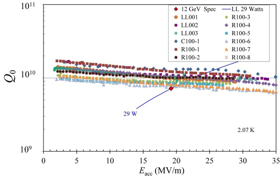
Figure 27. Performance of CEBAF 7-cell cavities after  $\sim 30 \mu\text{m}$  EP. From [146].
