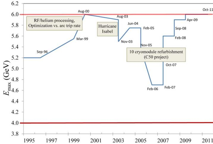
Figure 21. CEBAF maximum beam energy evolution prior to and during the C50 project.
