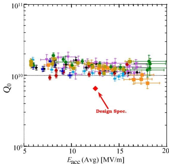
Figure 24. Acceptance test performance of cavities in the first intermediate prototype upgrade cryomodule (SL21) in the CMTF. From [118].
