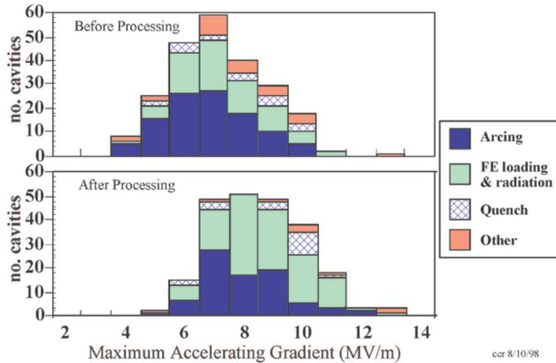
Figure 13. Cavity performance improvement with helium processing 1996-1998. From [85].
