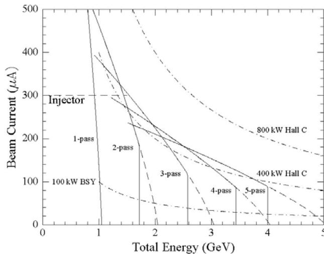
Figure 12. 1996 operational envelope of CEBAF at reduced klystron power. From [81].
