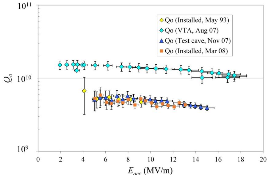
Figure 22. Performance of cavity IA-085 as installed in CEBAF in 1993, in reworked qualification VTA and cryomodule acceptance tests, and as recommissioned in CEBAF in 2008. From [106].
