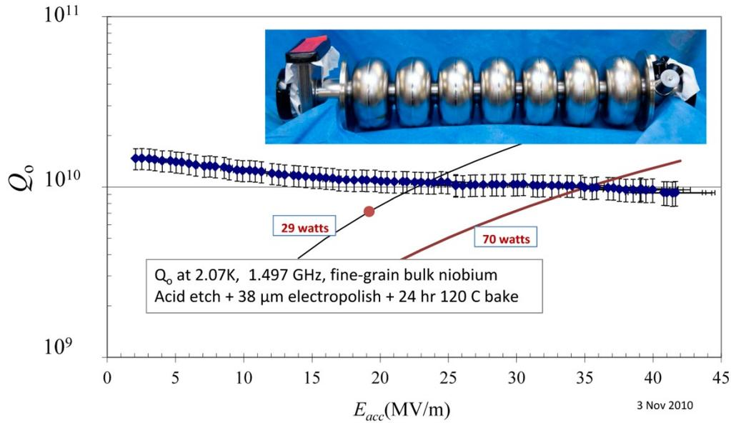
Figure 28. Performance test of cavity C100-6 without helium vessel.
