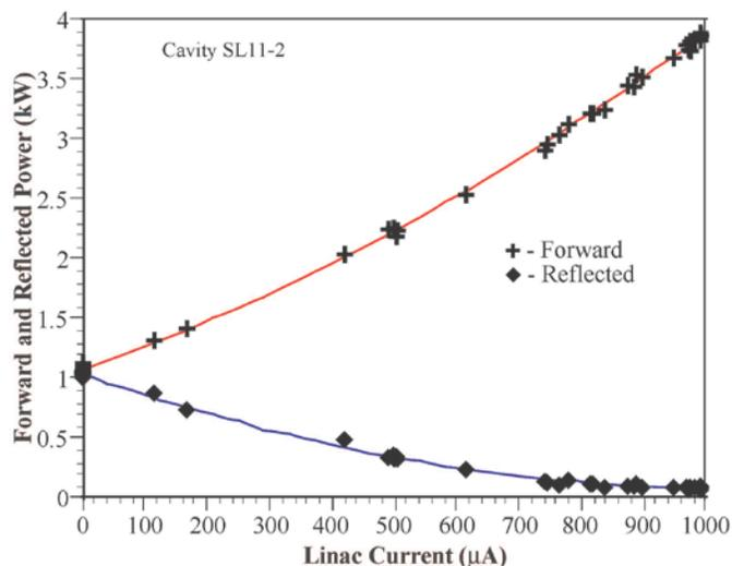
Figure 14. Matched RF load at full beam current. From [85].
