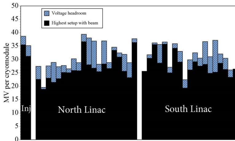
Figure 11. CEBAF available SRF cryomodule voltage in 1996. From [63].
