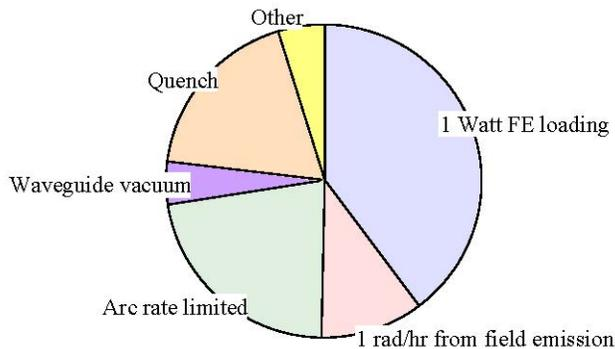
Figure 8. Distribution of CEBAF cavity gradient limitations, 1995. From [51].
