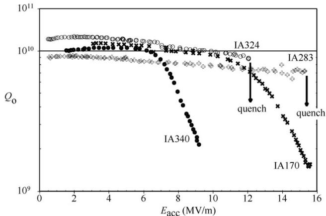
Figure 3. Representative performance of CEBAF cavities in 2 K acceptance tests. From [51].
