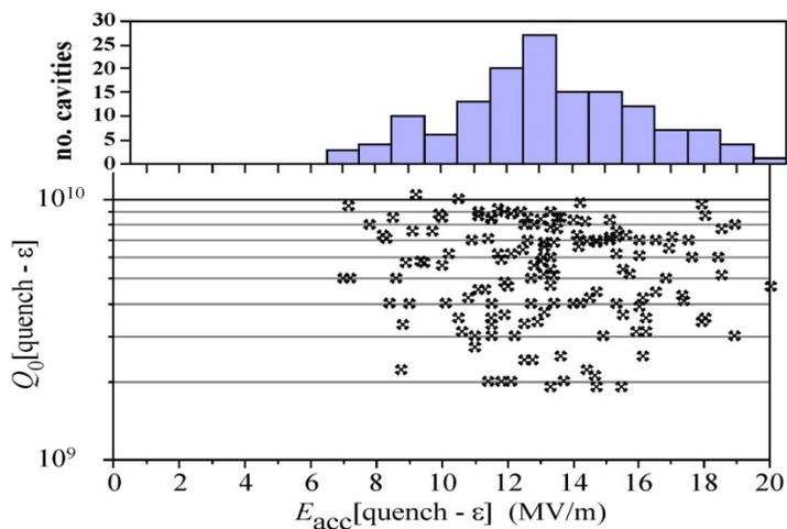
Figure 4. Cavity performance just below quench during pair testing. From [48].
