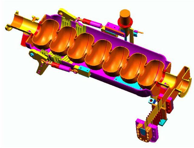
Figure 25. Cross-section of *Renascence* cavity, couplers, helium vessel, and tuner.
