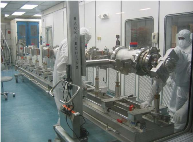
Figure 29. C100 cavity string assembly.
