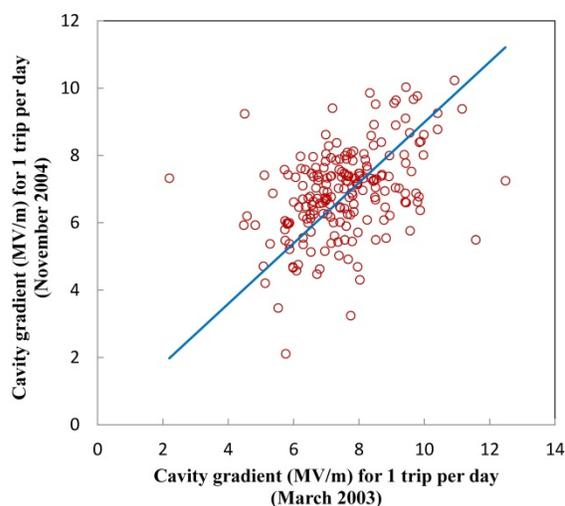
Figure 18. Comparison of fixed arc-rate gradient conditions before and after the hurricane-induced thermal cycle and recovery. From [90].
