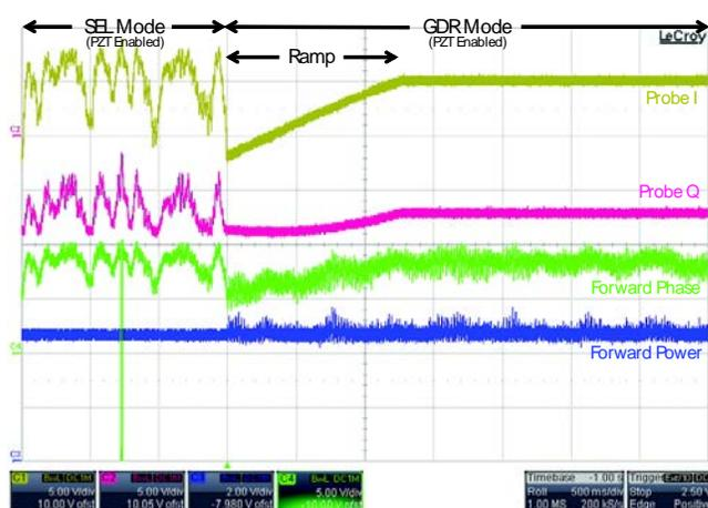
Figure 30. Annotated oscilloscope image capturing the transition from self-excited-loop (SEL) to generator-driven-resonator (GDR) control with piezotuner enabled. From [155].
