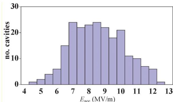
Figure 16. Distribution of cavity gradients producing 3 arcs per day. From [88].
