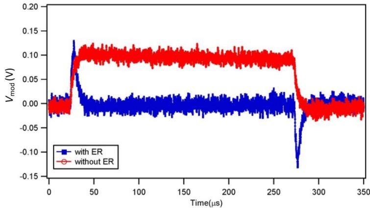
Figure 19. Forward power drive signal for an SRF cavity with 250  $\mu$ sec-duration tune beam with single beam (red) and a two-beam, energy recovering setup (blue). From [93].
