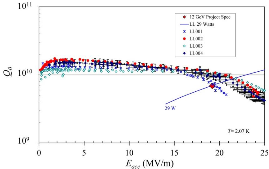
Figure 26. Qualification tests of the four Low Loss (LL) cavities for *Renascence*. From [123].
