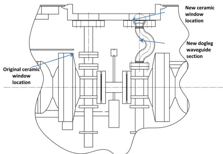
Figure 20. RF window relocation and dogleg waveguide in C50 cryomodules.
