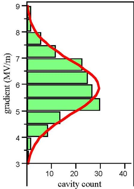
Figure 10. Modeled gradients for arc fault intervals of four days. From [70].
