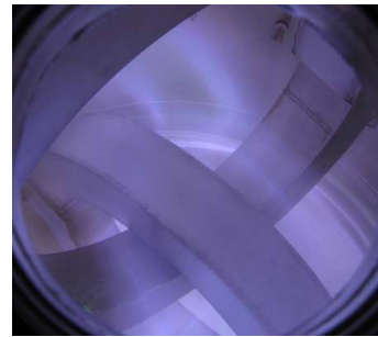
FIG. 2. Photograph of a typical argon plasma in CNT heated with 1 kW ECRH with CNT's two in-vessel coils in clear view.
