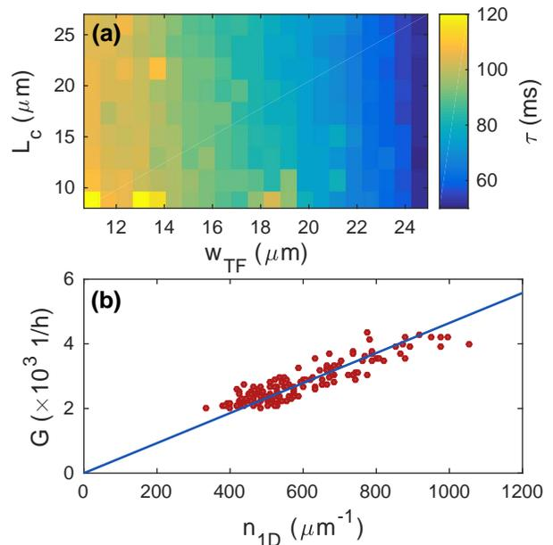
FIG. 4. (Color online) (a) Exponential decay time,  $\tau(L_c, w_{\text{TF}})$ , vs. the length of the channel  $L_c$  and the Thomas–Fermi width of the channel,  $w_{\text{TF}}$ . (b) Conductance  $G = 1/R$  vs. one-dimensional channel density,  $n_{1D}$ , with a linear fit.
