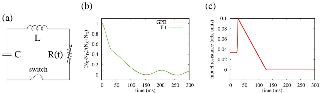
FIG. 1. (color online) (a) Model RLC circuit with variable resistance. (b) Number imbalance,  $\Delta N(t)$ , from the Gross–Pitaevskii (GP) equation and fitted result (see text) for a dumbbell potential with channel length  $L_c = 20 \mu\text{m}$  and Thomas–Fermi width of  $w_{\text{TF}} \approx 22 \mu\text{m}$ . (c) The time–dependent resistance,  $R(t)$ , derived from the fitted number imbalance.
