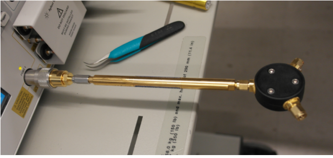
Fig. 7. Setup during measurements of the terminated airline. The black circular block at the end of the airline is a plastic holder for the three calibration standards.
