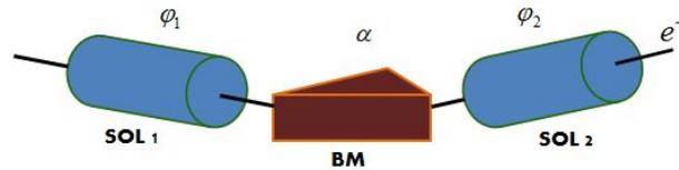
Figure 2.1: Elements of a Universal Synchronous Spin Rotator cell.
