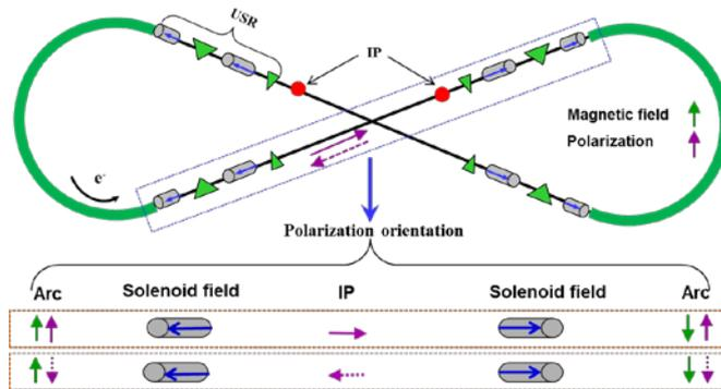
Figure 1.1: JLEIC electron polarization ( $\vec{S}$ , a purple arrow) directions remain the same in two arcs by having opposite longitudinal solenoid field directions in the same long straight. The blue arrow in a solenoid represents the field direction. The polarization orientation in one of the two long straights (shown in the blue dash-line box) is exhibited under the half brace with two different polarization states at the IP.
