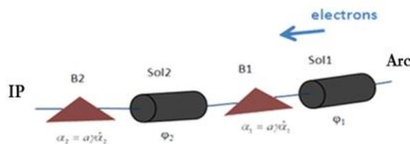
Figure 1.2: Universal Spin Rotator (USR) elements.
