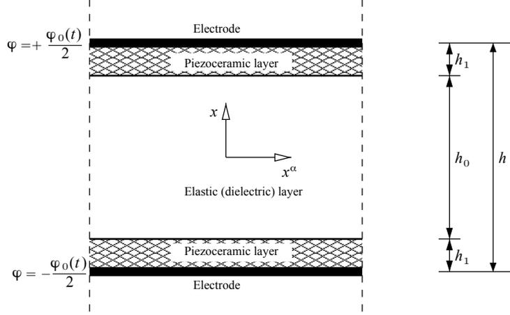
Figure 1: A side view of the sandwich shell
