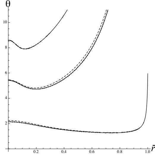
Figure 4: Three first resonant (bold lines) and anti-resonant frequencies (dashed lines) of the circular plate partially covered by piezoceramic rings versus  $\bar{r}$  at fixed  $\zeta_0 = 0.01$ .
