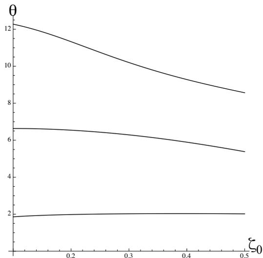
Figure 3: Three first resonant frequencies of the circular plate partially covered by piezoceramic rings versus the relative thickness  $\zeta_0$  at fixed  $\bar{r} = 0.5$ .
