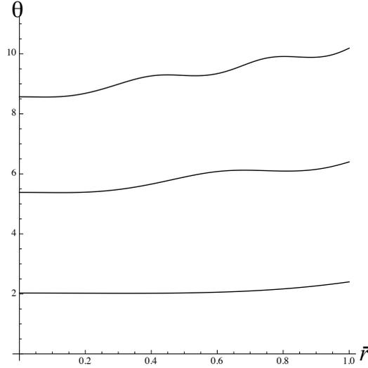
Figure 2: Three first resonant frequencies of the circular plate partially covered by piezoceramic rings versus the relative radius  $\bar{r}$  of the uncovered area at fixed  $\zeta_0 = 0.4$ .
