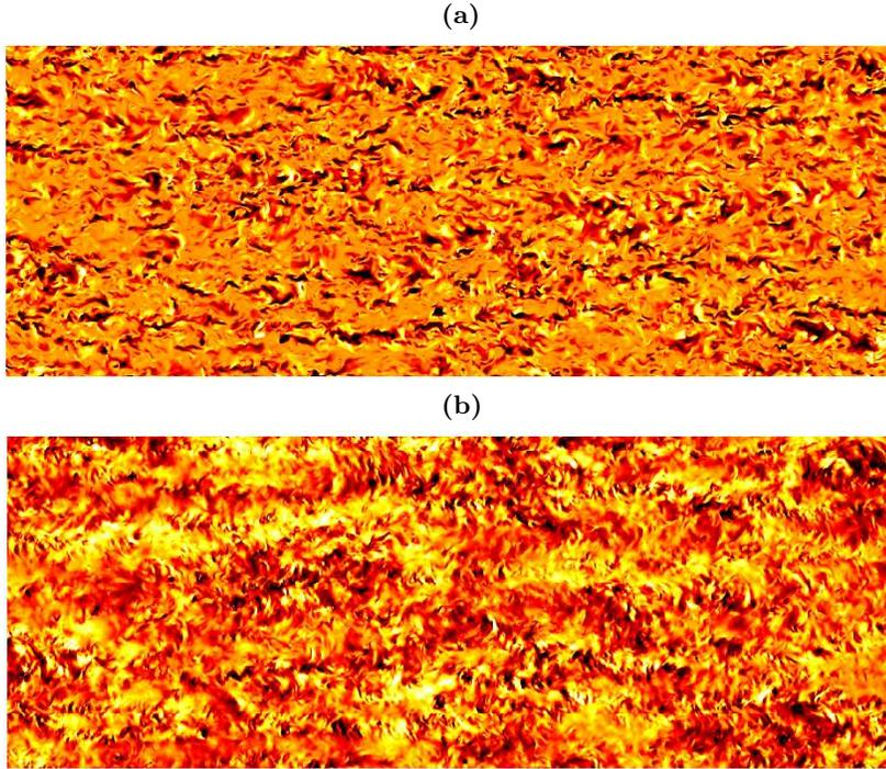
FIGURE 3. Wall-parallel snapshots of the instantaneous tangential momentum flux in a channel at  $Re_\tau = 934$  (del Álamo *et al.* 2004) and  $x_2/h = 0.15$ . Flow is from left to right, and the area in the figures is  $L_1 \times L_3 = 4\pi h \times 3\pi h/2$ . (a) Classical flux  $R'_{12}$  from eq:NS2bis. (b) Optimal flux  $\phi'_{12}$ . In both cases, the flux is centred with its mean value, and the colour scale spans  $\pm 3$  standard deviations, increasing from dark to light.
