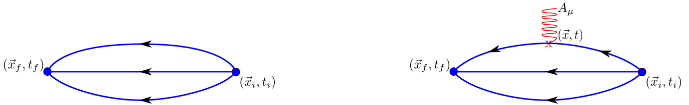
FIG. 2. The baryon two-point function (left) and the connected three-point function (right) are shown diagrammatically. The solid lines represent fully dressed quark propagators.
