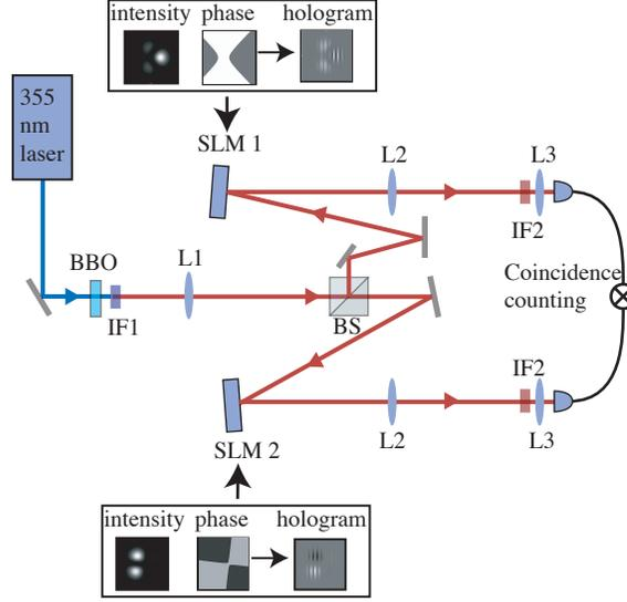
**Figure 2.** Experiment Setup. The holograms for measuring the states are programmed in SLMs. The insets show sample intensity and phase cross-sections of the measurement states and the holograms we use to measure. Black to white corresponds to: 0 to 1 for the normalised intensity, 0 to  $2\pi$  for the phase and 0 to 255 for the holograms.
