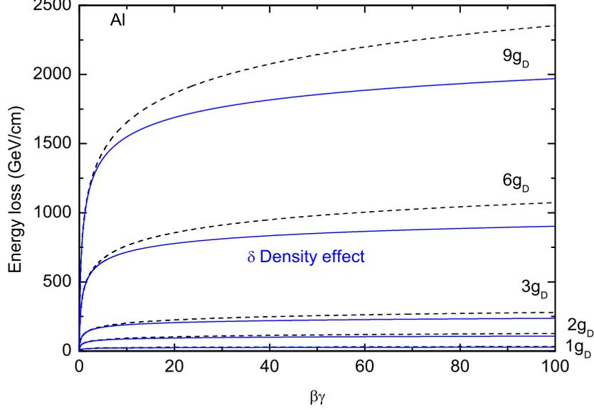
**Figure 2:** Energy loss of MMs in Aluminum vs  $\beta\gamma$  computed with (blue curves) and without (black dashed curves) the density effect correction taken into account. MMs of magnetic charges  $1g_D$ ,  $2g_D$ ,  $3g_D$ ,  $6g_D$  and  $9g_D$  are considered.
