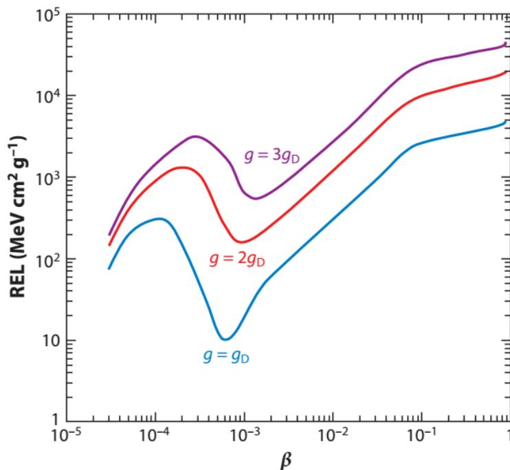
**Figure 13:** Restricted energy loss (REL) in CR39® vs  $\beta$  for  $1g_D, 2g_D$  and  $3g_D$  MMs. [12]
