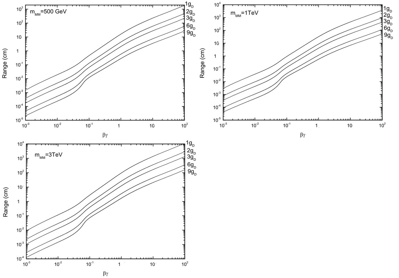
**Figure 10:** Ranges versus  $\beta\gamma$  in Aluminum for MMs with mass 0.5, 1 and 3 TeV and different magnetic charges ( $1g_D, 2g_D, 3g_D, 6g_D$  and  $9g_D$ ).
