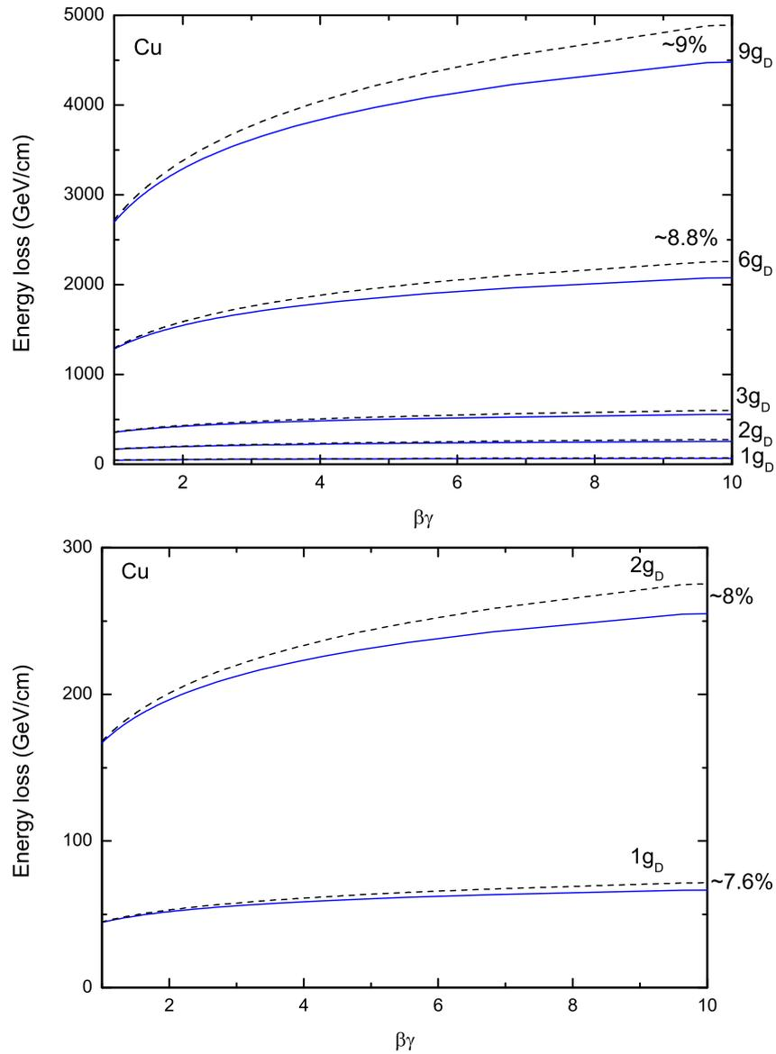
**Figure 5:** Energy loss of MMs in Copper vs  $\beta\gamma$  computed with (blue curves) and without (black dashed curves) the density effect correction taken into account for  $g = g_D$  and  $2g_D$  (bottom panel) and  $g = 3g_D, 6g_D$  and  $9g_D$  (top panel). Percentage values on the vertical scale (right) indicate the entity of the correction at  $\beta\gamma \sim 10$ .
