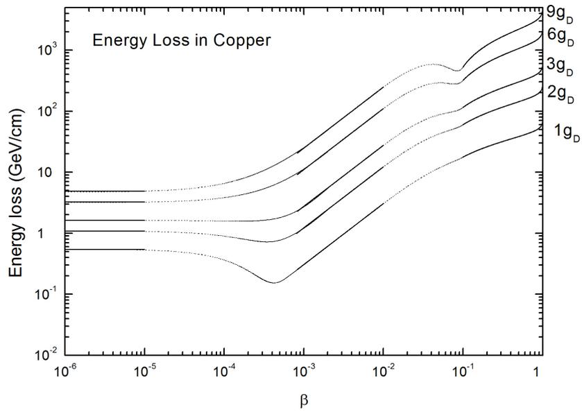
**Figure 8:** Energy loss of magnetic monopoles with charge  $1g_D$ ,  $2g_D$ ,  $3g_D$ ,  $6g_D$  and  $9g_D$  in Copper.
