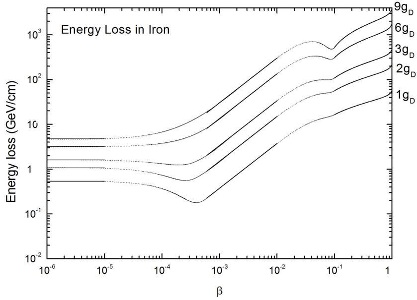
**Figure 7:** Energy loss of magnetic monopoles with charge  $1g_D$ ,  $2g_D$ ,  $3g_D$ ,  $6g_D$  and  $9g_D$  in Iron.
