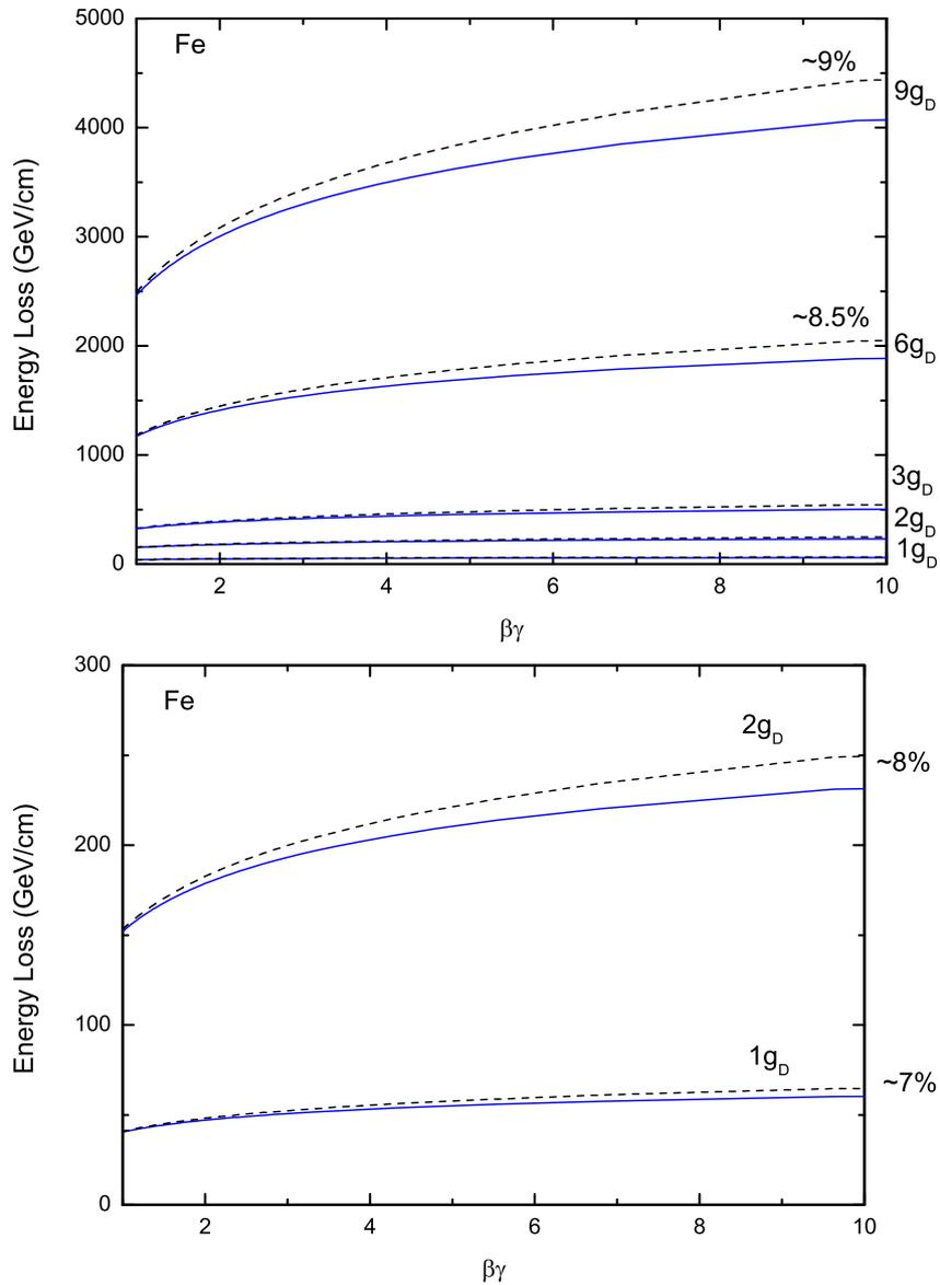
**Figure 4:** Energy loss of MMs in Iron vs  $\beta\gamma$  computed with (blue curves) and without (black dashed curves) the density effect correction taken into account for  $g = g_D$  and  $2g_D$  (bottom panel) and  $g = 3g_D$ ,  $6g_D$  and  $9g_D$  (top panel). Percentage values on the vertical scale (right) indicate the entity of the correction at  $\beta\gamma \sim 10$ .
