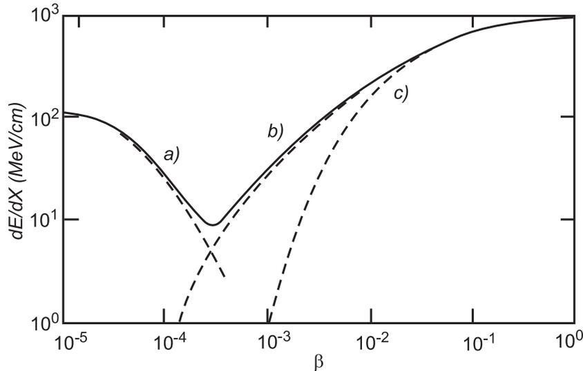
**Figure 1:** The energy losses, in MeV/cm, of  $g = g_D$  MMs in liquid hydrogen as a function of  $\beta$ . Curve a) corresponds to elastic monopole–hydrogen atom scattering; curve b) corresponds to interactions with level crossings; curve c) describes the ionization energy loss.
