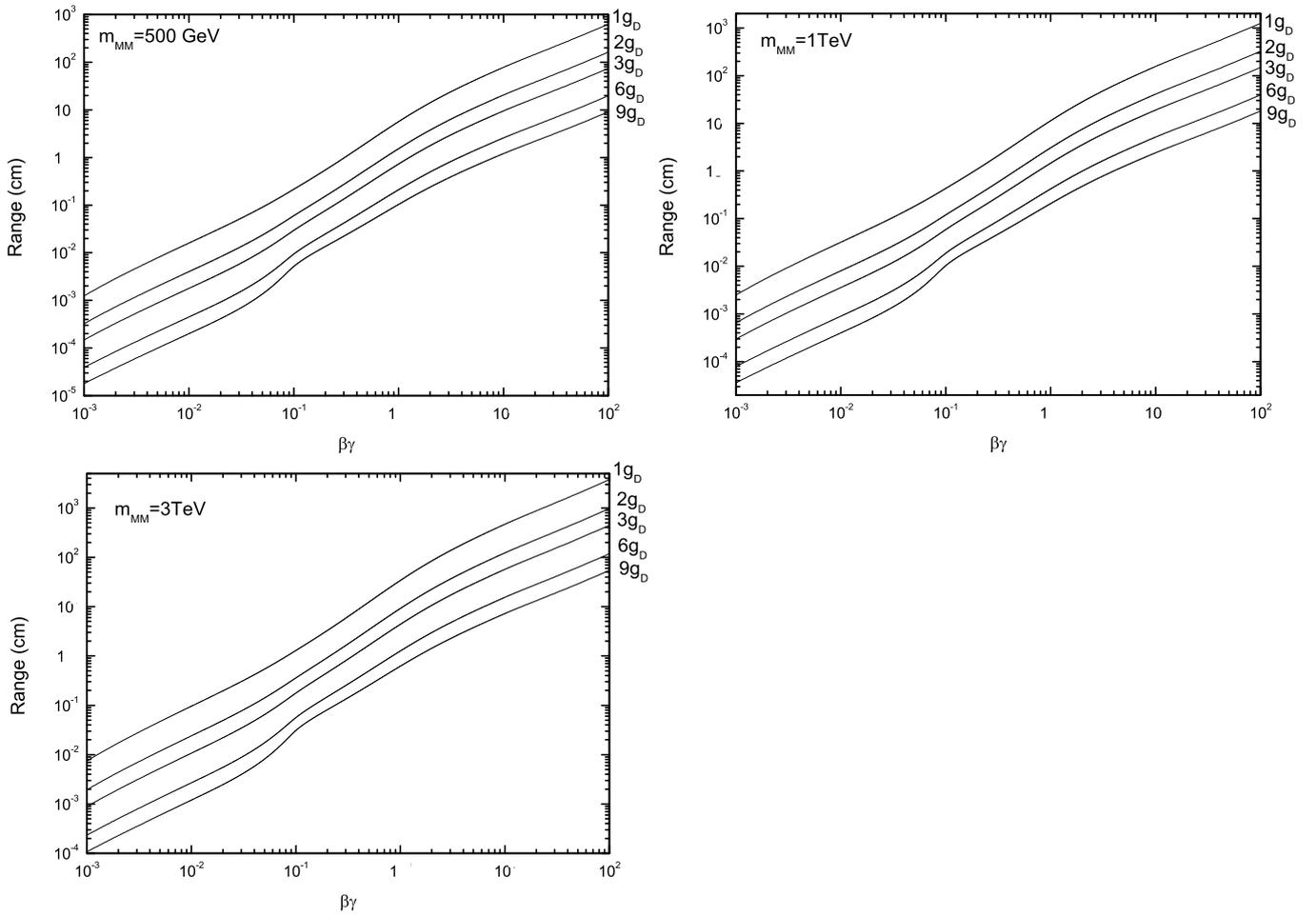
**Figure 12:** Ranges in Copper versus  $\beta\gamma$  for MMs with mass 0.5, 1 and 3 TeV and different magnetic charges ( $1g_D, 2g_D, 3g_D, 6g_D$  and  $9g_D$ ).
