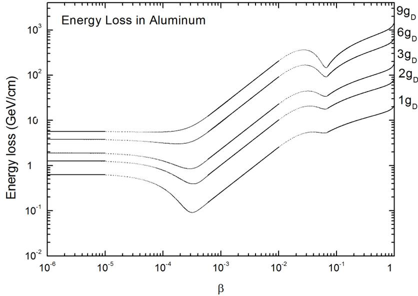
**Figure 6:** Energy loss of magnetic monopoles with charge  $1g_D, 2g_D, 3g_D, 6g_D$  and  $9g_D$  in Aluminum.
