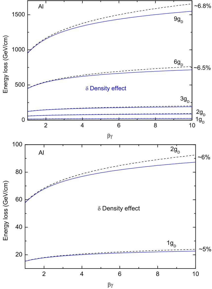
**Figure 3:** Energy loss of MMs in Aluminum vs  $\beta\gamma$  computed with (blue curves) and without (black dashed curves) the density effect correction taken into account for  $g = g_D$  and  $2g_D$  (bottom panel) and  $g = 3g_D$ ,  $6g_D$  and  $9g_D$  (top panel). Percentage values on the vertical scale (right) indicate the entity of the correction at  $\beta\gamma \sim 10$ .
