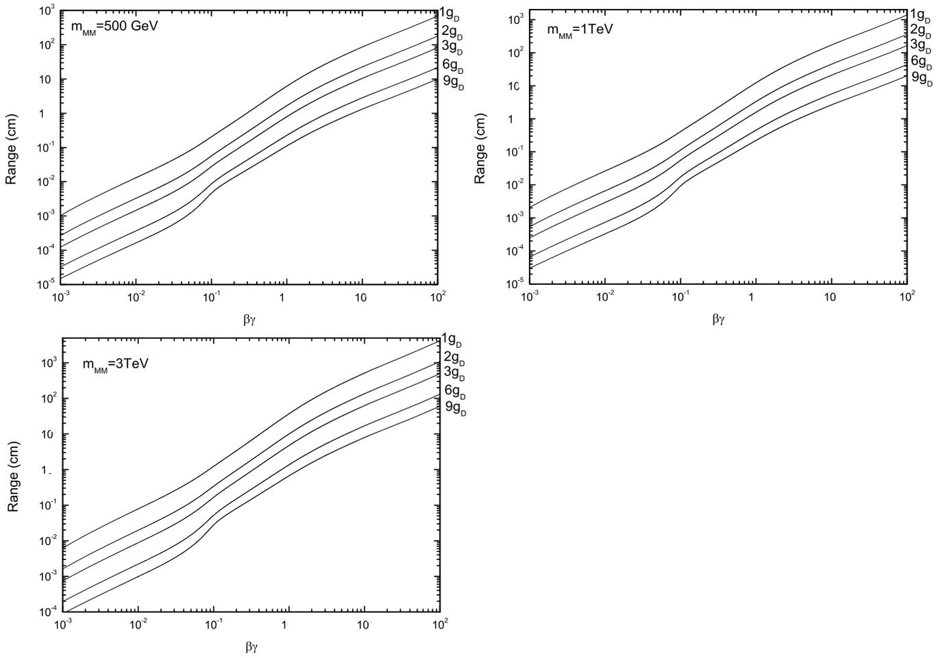
**Figure 11:** Ranges versus  $\beta\gamma$  in Iron for MMs with mass 0.5, 1 and 3 TeV and different magnetic charges ( $1g_D$ ,  $2g_D$ ,  $3g_D$ ,  $6g_D$  and  $9g_D$ ).
