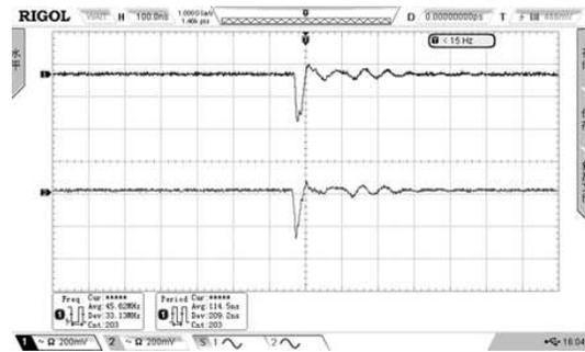
Fig. 8. The plastic scintillator response.
