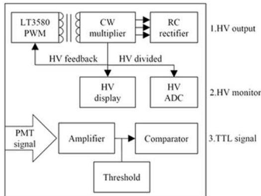
Fig. 2. Block diagram of the CW base.
