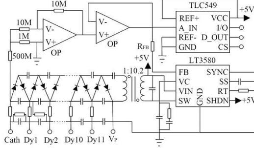
Fig. 4. Block diagram of high voltage supply and monitor.
