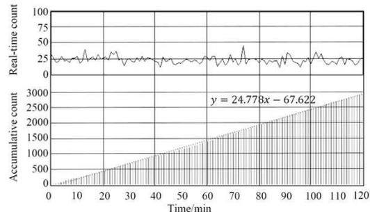
Fig. 11. Result of cosmic muon coincidence counting.
