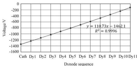
Fig. 6. The boost curves of PMT base.
