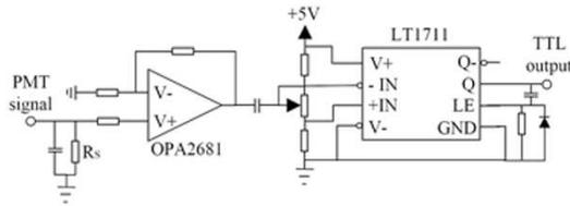
Fig. 5. Block diagram of signal processing circuit.
