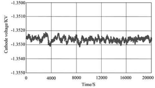
Fig. 7. A long-time stability test on cathode voltage.
