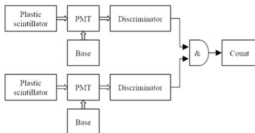
Fig. 10. Diagram of cosmic muon coincidence counting.
