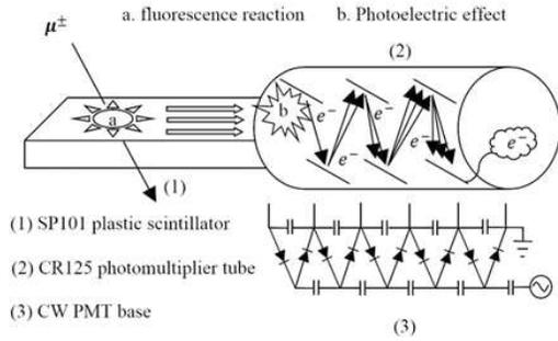
Fig. 1. Block diagram of the muon detector.
