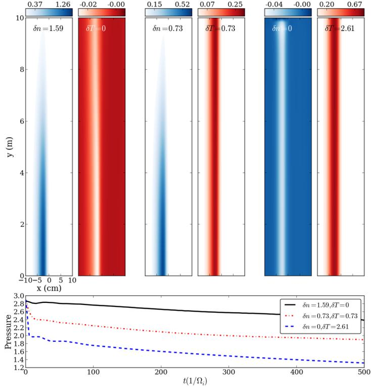
**Figure 10.** Upper row: Parallel profile of the density and temperature (with background profiles subtracted off) across each set of amplitudes in the constant pressure scan. The profiles are taken at  $t = 150/\Omega_i$ . Lower plot: Peak pressure in the filament at the midplane during the simulation. In the early phase a quick pressure drop occurs as electron conduction homogenises the temperature profile.
