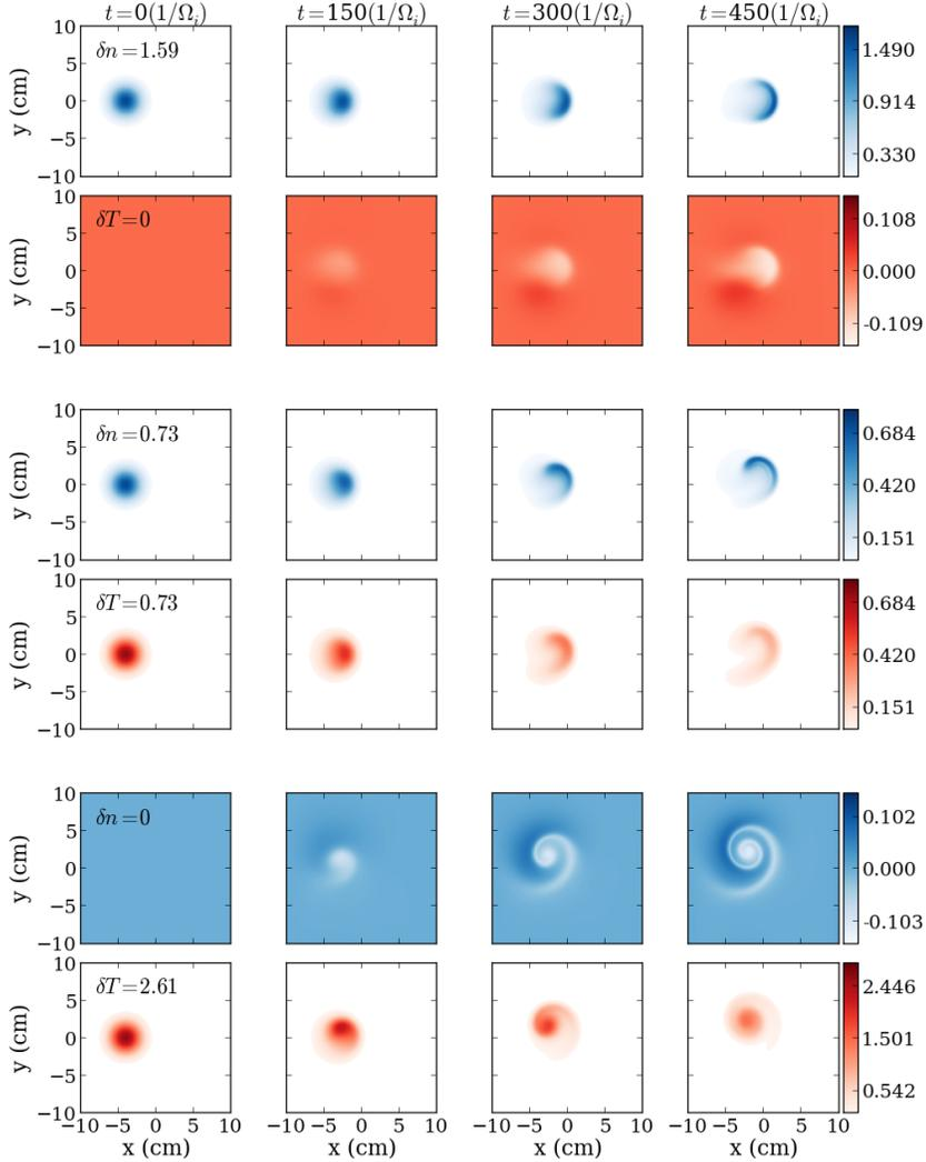
**Figure 2.** Cross sections of density (blue color scales) and temperature (red color scales) at the midplane shown at different points in the filament evolution. The three simulations corresponding to the three pairings of  $\delta n$  and  $\delta T$  given in (34) are shown.
