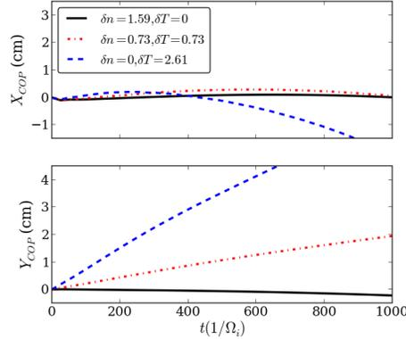
**Figure 13.** COM coordinate in the radial (upper) and bi-normal (lower) direction for the sheath limited filament with  $\delta_{\perp} = 8\text{cm}$  across the constant pressure scan in  $\delta n, \delta T$ .
