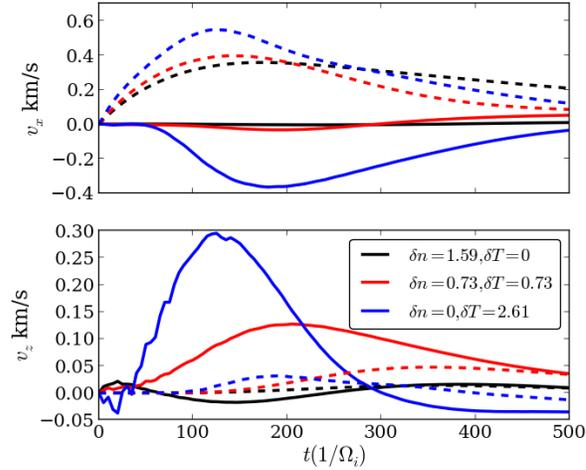
**Figure 6.** Cross-section averaged radial (upper) and bi-normal (lower) average  $\mathbf{E} \times \mathbf{B}$  velocity for the three cases in the constant pressure scan. Shown are contributions from the even (solid lines) and odd (broken lines) components of the potential.
