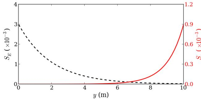
**Figure 14.** Source profiles used to create backgrounds for simulations run in this paper. The energy source (black broken line, left axis) and the particle source (red solid line, right axis) are shown as a function of parallel distance with  $y = 0$  at the midplane and  $y = L_{||} = 10\text{m}$  at the sheath.
