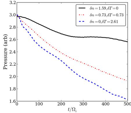
**Figure 8.** Maximum pressure in the filament at the midplane as a function of time for each combination of  $\delta n, \delta T$
