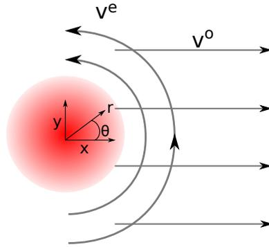
**Figure 7.** Schematic illustrating the geometry of the filament flow pattern with a constant flow in  $x$  of magnitude  $v^-$  and a circulatory flow in the positive  $\theta$  direction of magnitude  $v^+$ .
