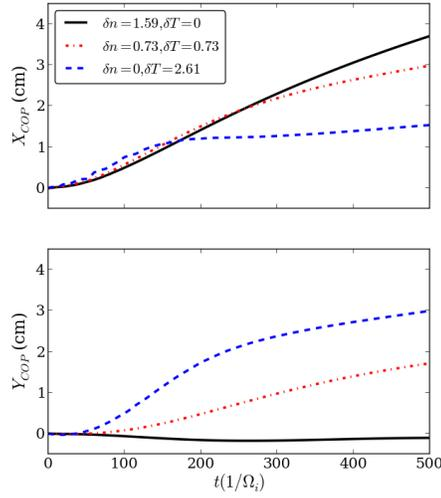
**Figure 4.** Centre-of-pressure position in the radial direction ( $x$ ) (upper) and in the bi-normal direction ( $z$ ) (lower) of the filament cross-section at the midplane in each of the simulations corresponding to the pairings of  $\delta n$  and  $\delta T$  given in (34).
