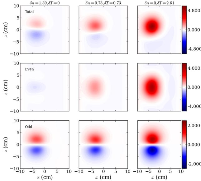
**Figure 3.** Electrostatic potential,  $\phi$  (upper row) and its even and odd components (middle and lower rows respectively) about the position of the filament centre in the bi-normal direction for each pair of amplitudes  $\delta n$  and  $\delta T$ . Profiles are shown at the midplane at  $t = 150/\Omega_i$  which is approximately at the maximum on the filament radial velocity.
