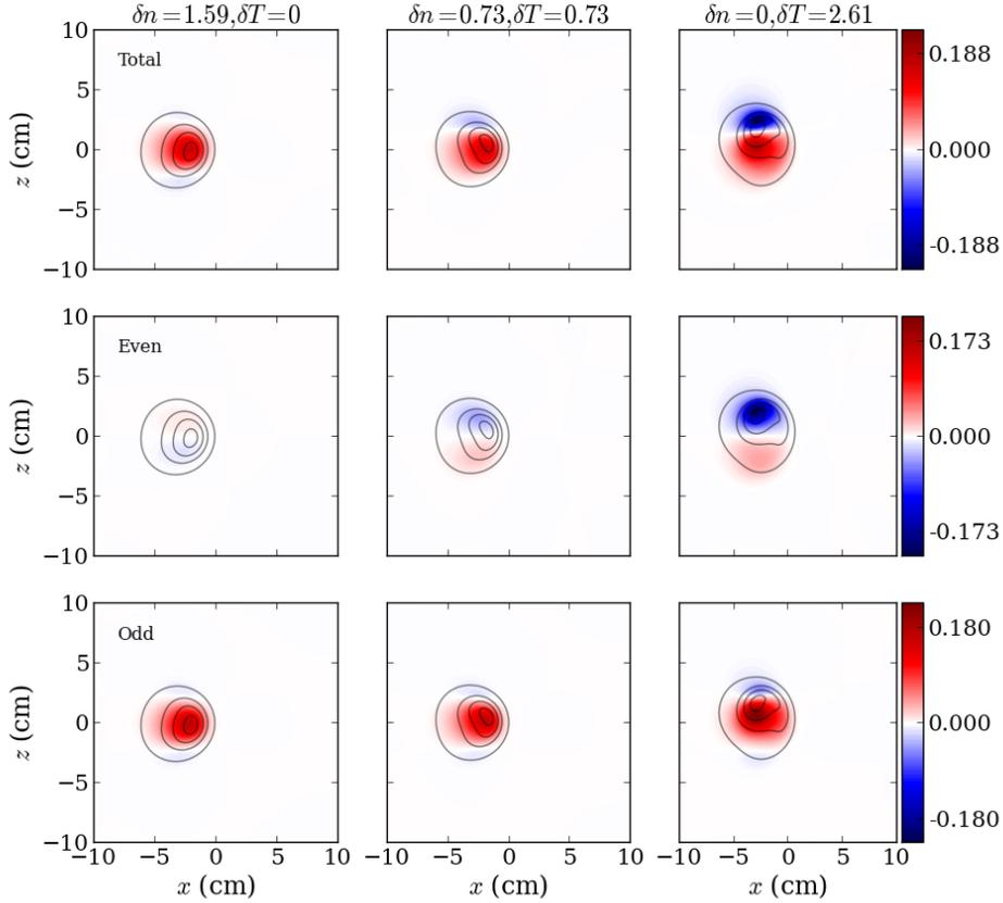
**Figure 5.** Radial  $\mathbf{E} \times \mathbf{B}$  heat flux from the total (upper), even (middle) and odd (lower) component of the potential at  $t = 150/\Omega_i$
