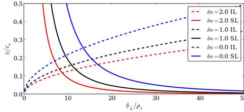
**Figure 1.** Scaling of the 2D filament characteristic velocity in the inertial regime (IL, broken lines) calculated from equation (30) and in the sheath limited regime (SL, solid lines) calculated from equation (31) for the following cases:  $\delta n = 2, \delta T = 0$  (red),  $\delta n = 1, \delta T = 1$  (black) and  $\delta n = 0, \delta T = 2$  (blue).
