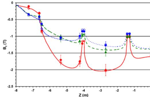
**Fig. 5** Axial magnetic flux density measured (*filled markers*) and calculated (*opened markers*) in the first (*rhombs*), second (*triangles*), and third (*circles*) barrel layers vs. Z-coordinate at the current of 19.14 kA. The *lines* represent the calculated values along the Hall sensors locations at the Y-coordinates of  $-4.805$  m (*solid line*),  $-5.66$  m (*dashed line*), and  $-6.685$  m (*dotted line*), corresponded to the first, second, and third barrel layer blocks, respectively
