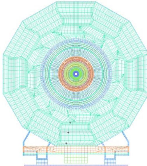
**Fig. 2** The  $XY$ -plane of the finite element mesh used to extrude the 3-D model. The *black crosses* near the azimuth angle of  $255^\circ$  display the location of the 3-D Hall sensors measured the magnetic flux density at the steel-air interfaces
