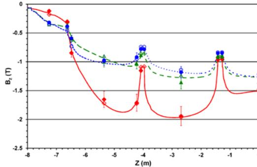
**Fig. 4** Axial magnetic flux density measured (*filled markers*) and calculated (*opened markers*) in the first (*rhombs*), second (*triangles*), and third (*circles*) barrel layers vs. Z-coordinate at the current of 17.55 kA. The *lines* represent the calculated values along the Hall sensors locations at the Y-coordinates of  $-4.805$  m (*solid line*),  $-5.66$  m (*dashed line*), and  $-6.685$  m (*dotted line*), corresponded to the first, second, and third barrel layer blocks, respectively
