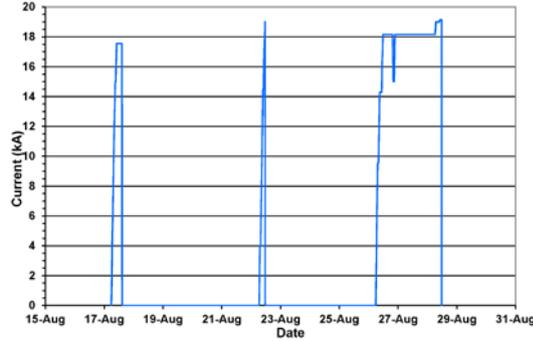
**Fig. 3** The CMS magnet current cycles of August 2006 used in the flux loops and 3-D Hall sensors measurements at 17.55 kA (17-Aug) and 19.14 kA (28-Aug)
