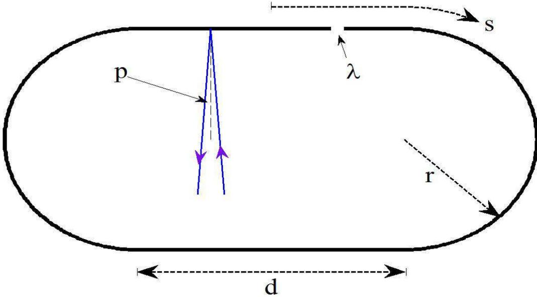
FIG. 1. The Bunimovich stadium with a leak of width  $\lambda$ . When a particle trajectory collides with a straight edge with a  $p$  value close to 0 we say that the particle is in a Marginally Unstable Periodic Orbit (MUPO). Such particles will progress slowly along the straight edges.
