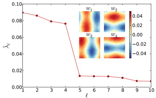
Figure 4: Explained variance ratios of the COP Ising model. Insets show the weights corresponding to the four leading principal components.
