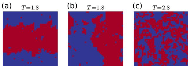
Figure 3: Typical configurations of the COP Ising model at below (a,b) and above (c) the critical temperature. Red and blue pixels indicate up and down spins. There are exactly half of the pixels are red/blue due to the constraint  $\sum_i \sigma_i \equiv 0$ .
