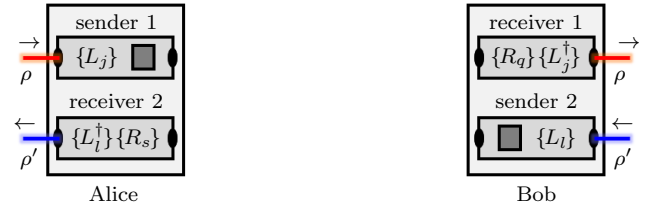
FIG. 12: (color online) Two-way ansible. Alice sends a message as \rho into sender 1, which comes out as \rho from Bob’s receiver 1. Bob uses tomography and obtains Alice’s message from \rho and then sends his response as \rho' into sender 2, and it comes out as \rho' from Alice’s receiver 2, where she can obtain Bob’s message from \rho' through tomography.
