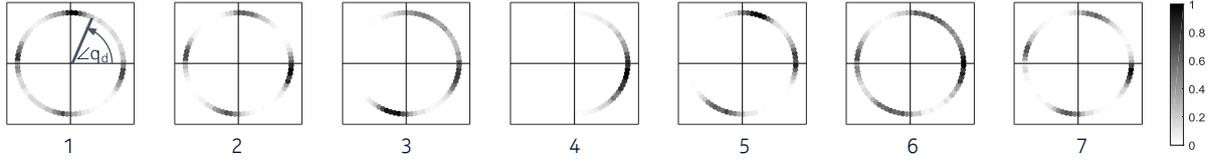
**Fig. 4:** Histograms (2800 symbols) of spectral amplitude phases  $\angle q_d(\lambda_i)$  of eigenvalues  $\lambda_i$  ( $i=1\dots 7$ ) measured at transmitter. Gray scale denotes relative occurrence.
