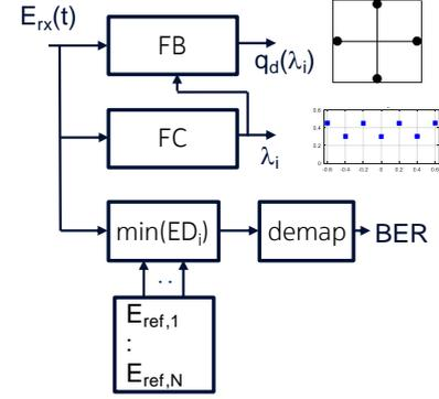
**Fig. 2:** Offline processing of received 2-ns signal traces  $E_{rx}(t)$ . FB:  $q_d$  by a forward-backward NFT algorithm. FC:  $\lambda_i$  by Fourier collocation method.  $\min(ED)$ : Decision on min. Euclidian distance.
