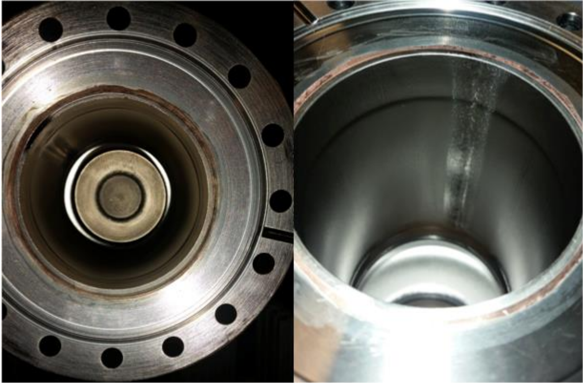
FIG. 3. The images of single cell cavity plasma etched (left) and buffer chemical polished (right).
