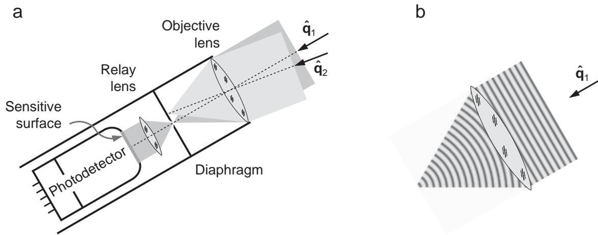
**Fig. 8.** Optical scheme of a well-collimated radiometer.
