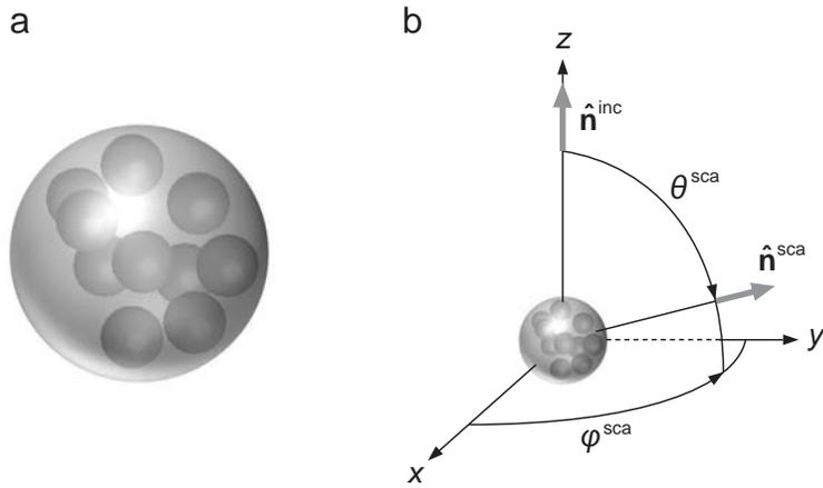
**Fig. 14.** (a) Model compound scatterer. (b) Scattering geometry.
