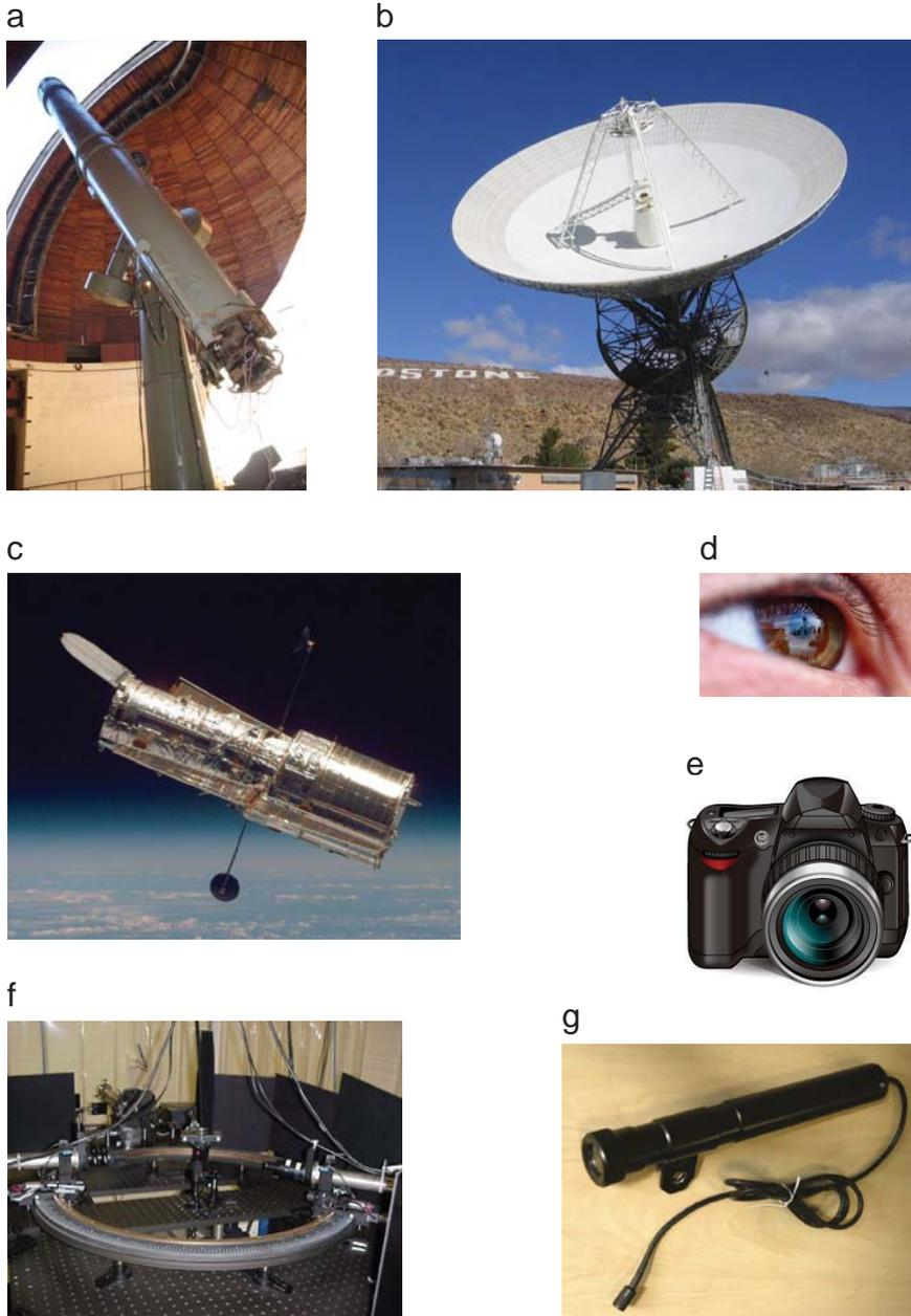
**Fig. 9.** Examples of well-collimated radiometers. (a) 26-in refractor of the Pulkovo Observatory. (b) NASA’s 34-m Goldstone radio telescope. (c) NASA’s Hubble Space Telescope. (d) Human eye. (e) Digital photographic camera. (f) Light scattering setup built at the University of Amsterdam (after [176]). (g) Gershun tube (after [177]).
