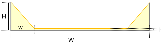
FIGURE 16. Simplified schematic diagram of the shape taken by the membrane for very high levels of collapse. The depth h of the thin liquid layer in the centre of the channel is below experimental resolution. Distances on the vertical axis have been stretched by a factor 6 for clarity.
