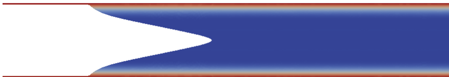
FIGURE 13. Shape of a symmetric finger obtained by finite-element simulations (using the oomph-lib library) in a depth-averaged model of air finger propagation in a rigid channel of spatially varying depth. Colours map the relative local channel depth, which has been chosen to mimic the membrane profile at very high collapse. The capillary number is Ca=0.47 .
