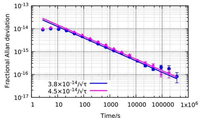
**Figure 4.** Fractional Allan deviation of the frequency comparison between the Sr2 clock and the FO2 dual fountain using Cs (blue ●) simultaneously with Rb (pink ▲) over ten days (October 2014). The stability is limited by the quantum projection noise of the fountain, and reaches a statistical resolution below  $10^{-16}$  after a few days of measurement.
