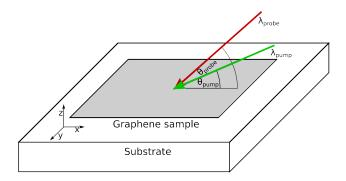
FIG. 1. The coordinate system under consideration. Two beams of wavelengths  $\lambda_{pump}$  and  $\lambda_{probe}$  are incident on a graphene sample on a quartz substrate, impinging with angles  $\theta_{pump}$  and  $\theta_{probe}$ , respectively.
