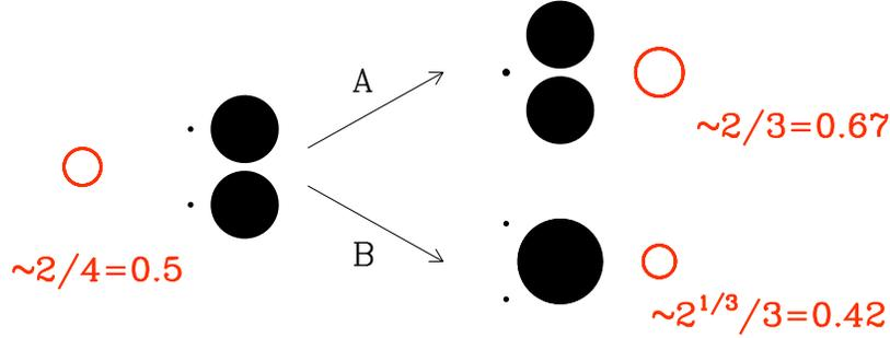
**Figure G.1.** Sketch illustrating the growth of  $\bar{r}$  when two small particles collide (A) and the decrease of  $\bar{r}$  when two large particles collide (B). Filled black symbols denote actual particle sizes and open red symbols and red text refer to  $\bar{r}$ .
