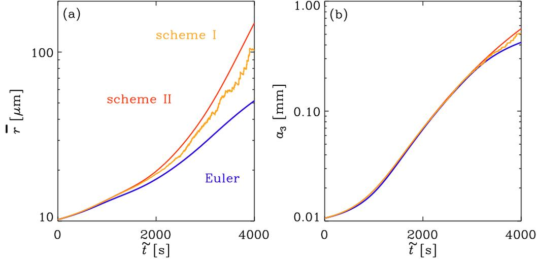
**Figure 2.** 3-D simulations with the swarm model and  $32^3$  grid points using schemes II (red) and I (orange), compared with the Eulerian model with  $\beta = 128$  (solid blue line) for (a)  $\bar{r}$  and (b)  $a_3$ . The collection is driven by gravity. See Runs 3C, 4B, and 6A of Table 1 for simulation details.
