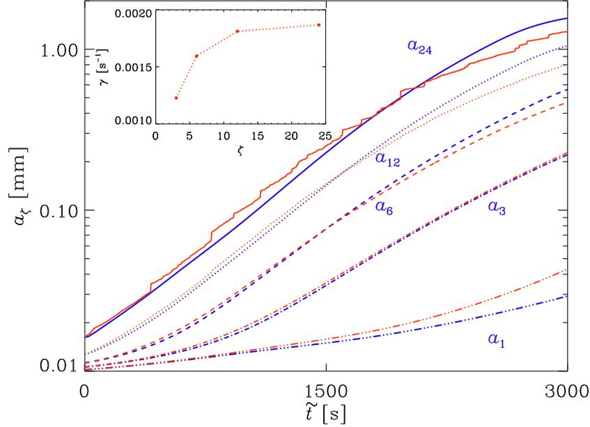
**Figure 4.** Same simulations as in Figure 2, but here we only compare the scheme II and the Eulerian model. Time evolution of  $a_1$  (three-dotted dashed line),  $a_3$  (dash-dotted lines),  $a_6$  (dash lines),  $a_{12}$  (dotted lines), and  $a_{24}$  (solid lines) of the size spectra are given. The inset shows the growth rates, for several moments (fitted between  $r=50 \mu\text{m}$  and  $r=200 \mu\text{m}$ ).
