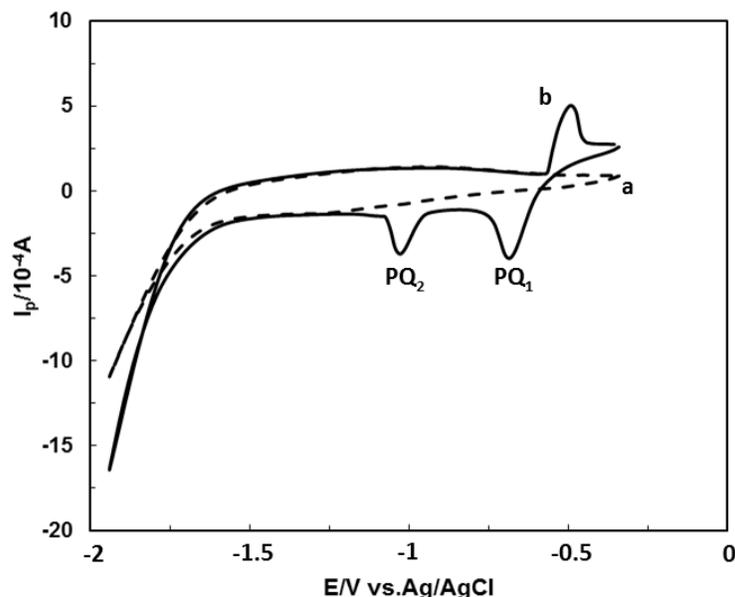
**Fig 3.** Cyclic voltammograms of  $9 \times 10^{-3}$  M PQ at (a) non-imprinted Ppy/EBB/GPE and (b) imprinted-Ppy/EBB/GPE in phosphate buffer at pH 7.0 with 0.2 M KCl.
