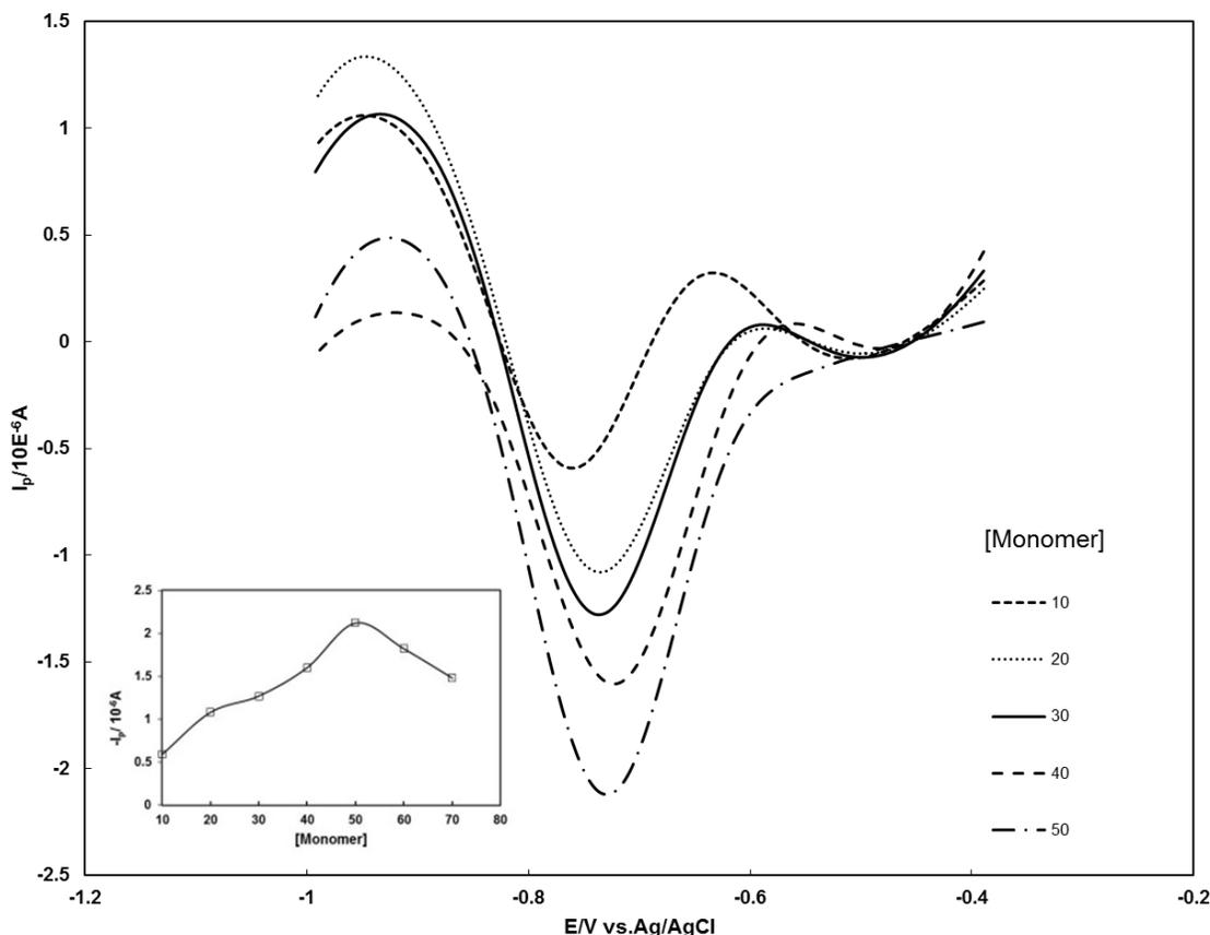
**Fig 5.** Differential pulse voltammogram of 30  $\mu\text{M}$  PQ at the imprinted Ppy/EBB/GPE in phosphate buffer at pH 7.0 with 0.2 M KCl for different monomer concentrations
