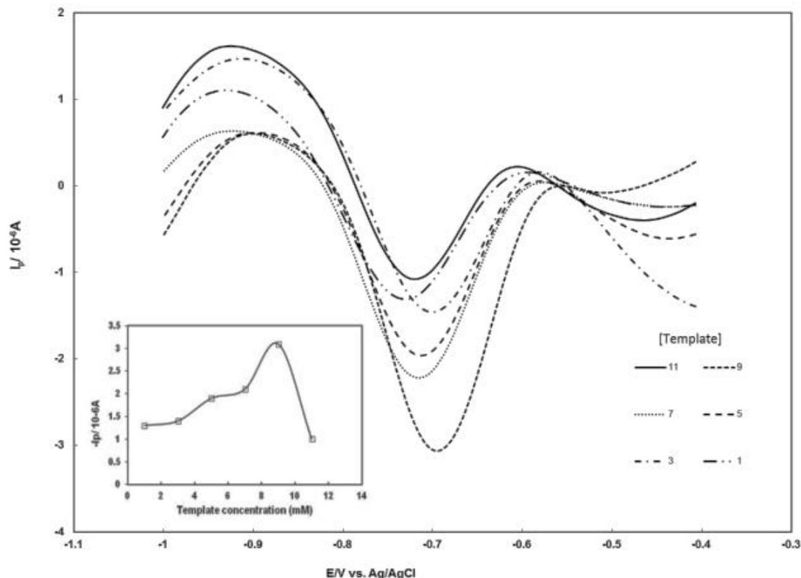
**Fig 4.** Current response diagram of 30  $\mu\text{M}$  PQ at the imprinted Ppy/EBB/GPE in phosphate buffer at pH 7.0 with 0.2 M KCl for different template concentrations
