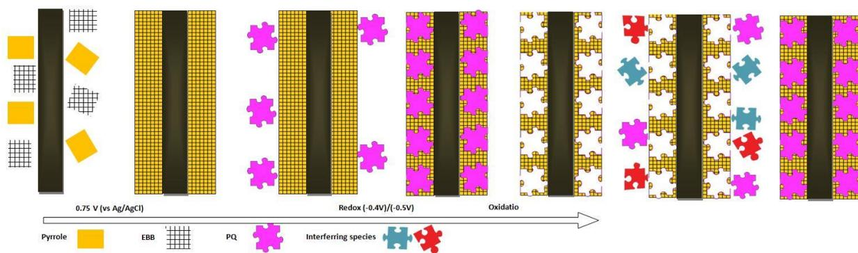
**Fig. 1** Schematic illustration of the fabrication of imprinted Ppy/EBB/GPE
