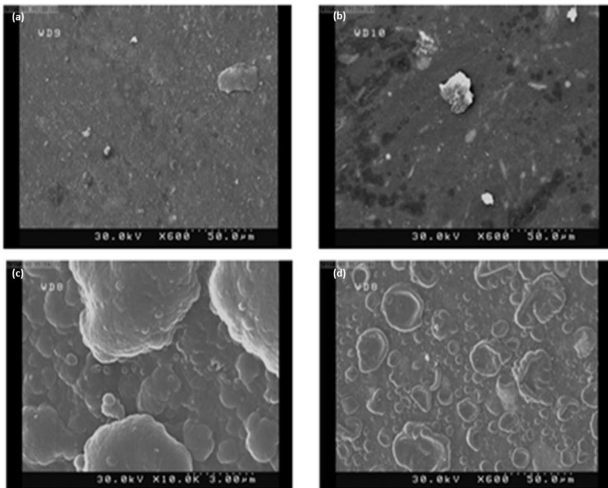
**Fig 2.** SEM micrographs of: (a) GPE, (b) non-templated, (c) templated by Ppy/EBB/GPE, (d) templated by Ppy/EBB/GPE before extracting the template
