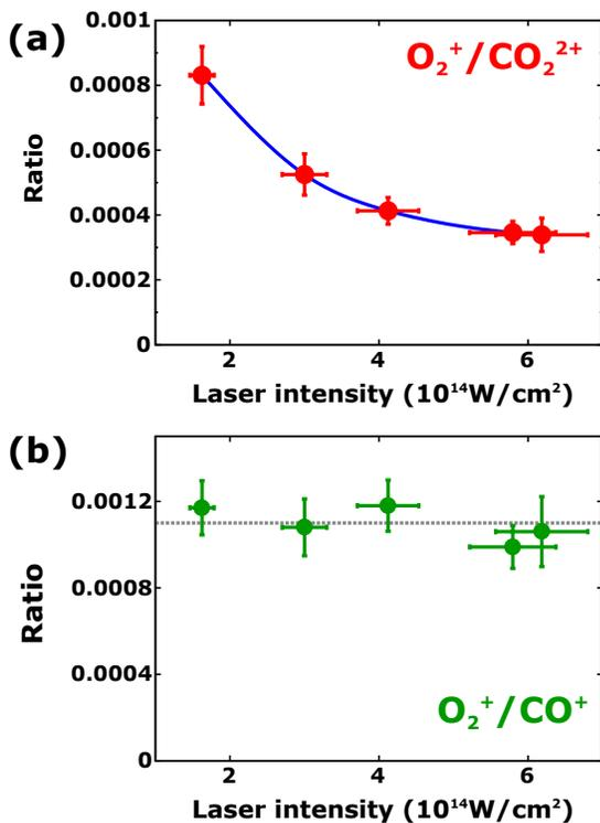
FIG. 4. (a) Ratio between the yields of  $\text{O}_2^+$  and that of stable  $\text{CO}_2^{2+}$  as a function of the laser peak intensity. (b) Ratio between the yields of  $\text{O}_2^+$  and  $\text{CO}^+$  channels as a function of the laser peak intensity. The blue line in (a) and the gray line in (b) are used to guide the eyes.
