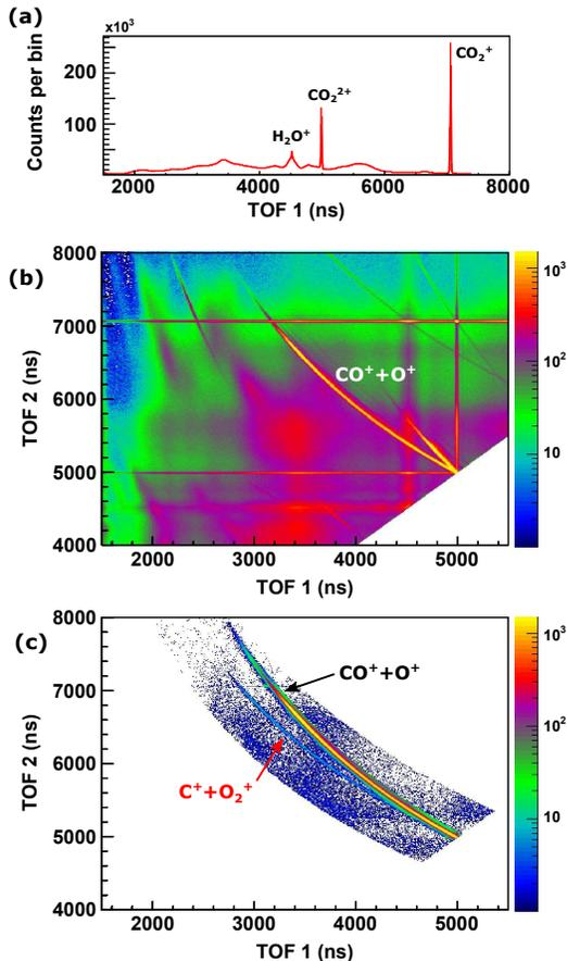
FIG. 1. (a) Measured time-of-flight spectrum of ions. (b,c) Measured photo-ion-photo-ion coincidence distribution without (b) and with (c) coincidence selection.
