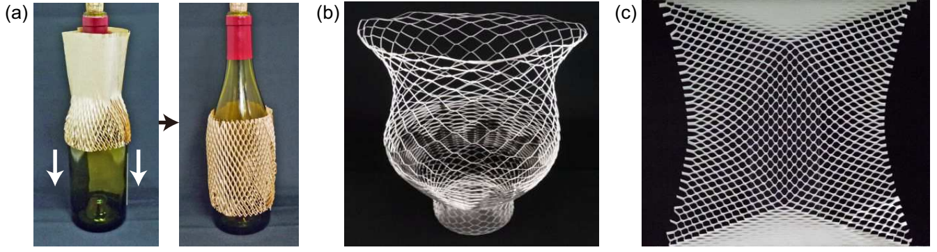
Figure 1. (a) A sheet of paper perforated with many cuts, kirigami , used for the protection of a bottle of wine. (b) "Airvase" (Trafu Architects, Japan) sold in museum shops worldwide, made from a sheet of kirigami. (c) Planer stretching of a sheet of kirigami with similar perforation geometry. The lack of circular symmetry leads to inhomogeneously stretched cuts.
