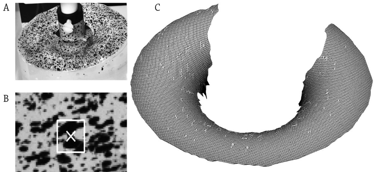
Figure 1: (A) The silicone gel phantom model and piston, (B) Close-up of speckles showing a subset, (C) A Delaunay triangulation of the tracked data points on the gel surface
