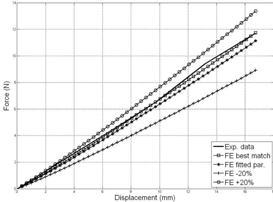
Figure 5: Indentor force displacement curves. Experimental (solid), FE best match to experimental (solid, square), FE using fitted parameters (solid, star), FE using 20% lower  $\mu$  (solid, plus), FE using 20% higher  $\mu$  (solid, circle).
