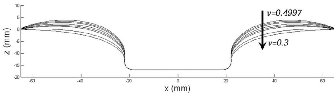
Figure 4: Influence of choice of Poisson's ratio on resulting FE deformation at piston depth of 16.74mm. From top to bottom surface deformation for  $\nu=0.4997$  (best match),  $\nu=0.495$ ,  $\nu=0.49$ ,  $\nu=0.48$ ,  $\nu=0.47$ ,  $\nu=0.45$ ,  $\nu=0.4$  and  $\nu=0.3$ .
