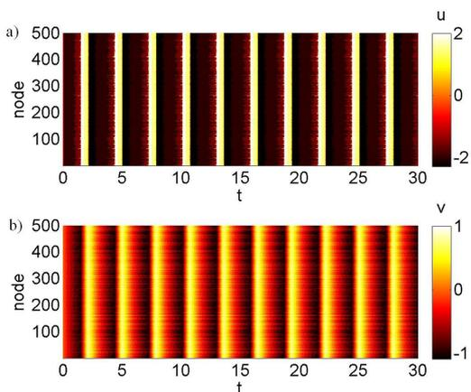
FIG. 13. Control of synchronization in 500 FitzHugh-Nagumo systems with a random topology by external stimulus  $I(t)$  according to Eqs. (27) and (28). (a) and (b): time series of the activator and the inhibitor of all nodes, respectively. Parameters:  $\gamma = 0.3$ ,  $a = 0.9$ . Other parameters and initial conditions as in Fig. 12
