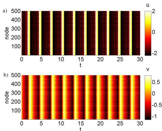
FIG. 9. Control of synchronization in 500 FitzHugh-Nagumo systems with a locally coupled ring topology Eq. (26) by the external stimulus  $I(t)$  according to Eqs. (27) and (28). (a) and (b): time series of the activator and the inhibitor of all nodes, respectively. Parameters:  $\gamma = 0.3$ ,  $a = 0.9$ . Other parameters and initial conditions as in Fig. 8.
