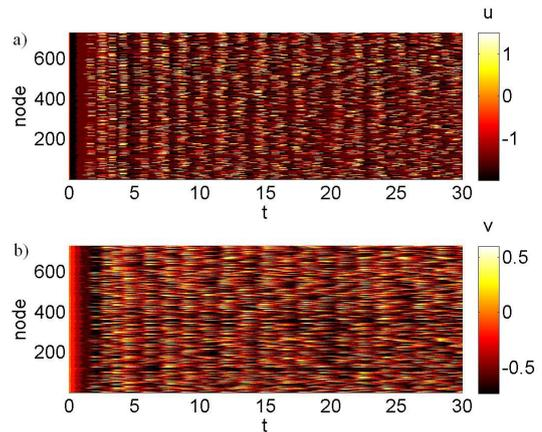
FIG. 10. Dynamics of 730 FitzHugh-Nagumo systems with Cantor-type hierarchical topology without control, i.e.,  $I(t) = 0$ . (a) and (b): time series of the activator and the inhibitor of all nodes, respectively. Parameters:  $n = 6$ ,  $N = 730$ ,  $C = 0.001$ . Other parameters and initial conditions as in Fig. 1.
