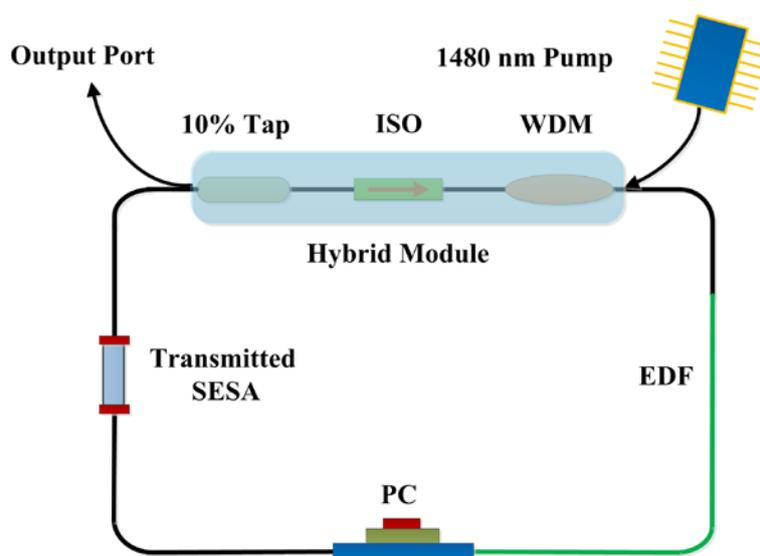
Fig. 1. Schematic of the passively mode-locked EDFL.
