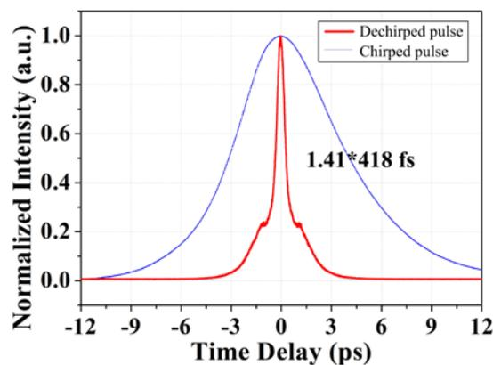
Fig. 3. Autocorrelation traces of the chirped and dechirped pulses.
