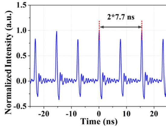
Fig. 4. Oscilloscope trace of the period-doubling of DSs.
