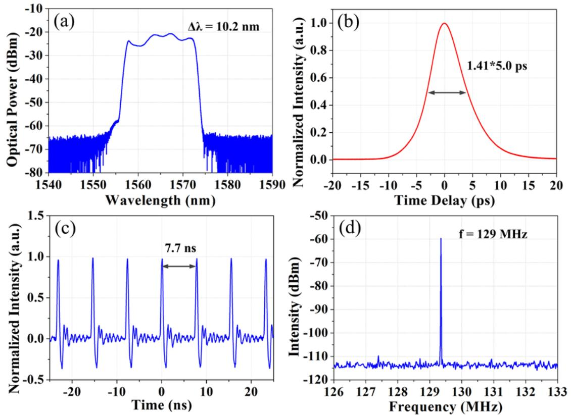
Fig. 2. (a) Optical spectrum, (b) autocorrelation trace, (c) oscilloscope trace, and (d) RF spectrum of the 129 MHz fundamental mode-locked DSs.
