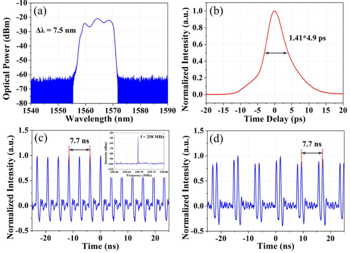
Fig. 5. (a) Optical spectrum, (b) autocorrelation trace and (c) oscilloscope trace of the 2nd-order harmonic mode-locked DSs (inset of Fig. 5(c) is the corresponding RF spectrum); (d) oscilloscope trace of the period-doubling of dual DSs.
