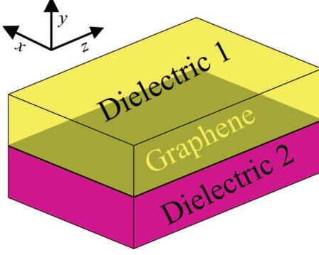
FIG. 1: (Color Online) Schematic of the structure, where the graphene layer is placed on the  $xz$  plane, and sandwiched by the dielectric 1 (yellow area) and dielectric 2 (pink area). The permittivities and permeabilities of the two dielectrics are  $(\varepsilon_1, \mu_1)$  and  $(\varepsilon_2, \mu_2)$ , respectively.
