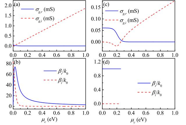
FIG. 2: (Color Online) Top row: The dependence between the surface conductivity and the chemical potential, where  $\sigma_{g,r}$  is the real part of surface conductivity, and  $\sigma_{g,i}$  is the imaginary part. Bottom row: The dependence between the propagation constant and the chemical potential, where  $\beta_r$  is the real part of propagation constant, and  $\beta_i$  is the imaginary part. The incident frequency is  $f = 10$  THz for (a)-(b) and  $f = 100$  THz for (c)-(d).
