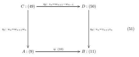
It turns out that the superposition of the three linearizable transformations shown in the picture can be rewritten as (10) which is of the form (2):  $\eta = \eta_3 \circ \eta_2 \circ \eta_1^{-1}$ .
