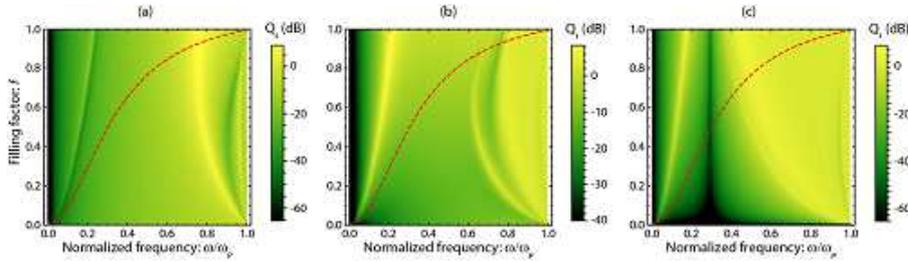
**Fig. 7** Scattering efficiency, expressed in dB, of a cylindrical cavity of radius  $R = k_p^{-1}/2$  and thickness  $T = R/2$ , when varying the dielectric constant of the core and environment medium: (a)  $\epsilon_C = 10$  and  $\epsilon = 1$ , (b)  $\epsilon_C = 1$  and  $\epsilon = 10$ , and (c)  $\epsilon_C = 10$  and  $\epsilon = 10$ . The red dashed line corresponds to frequencies  $\omega_{zero}$  which are solutions to the equation (18).
