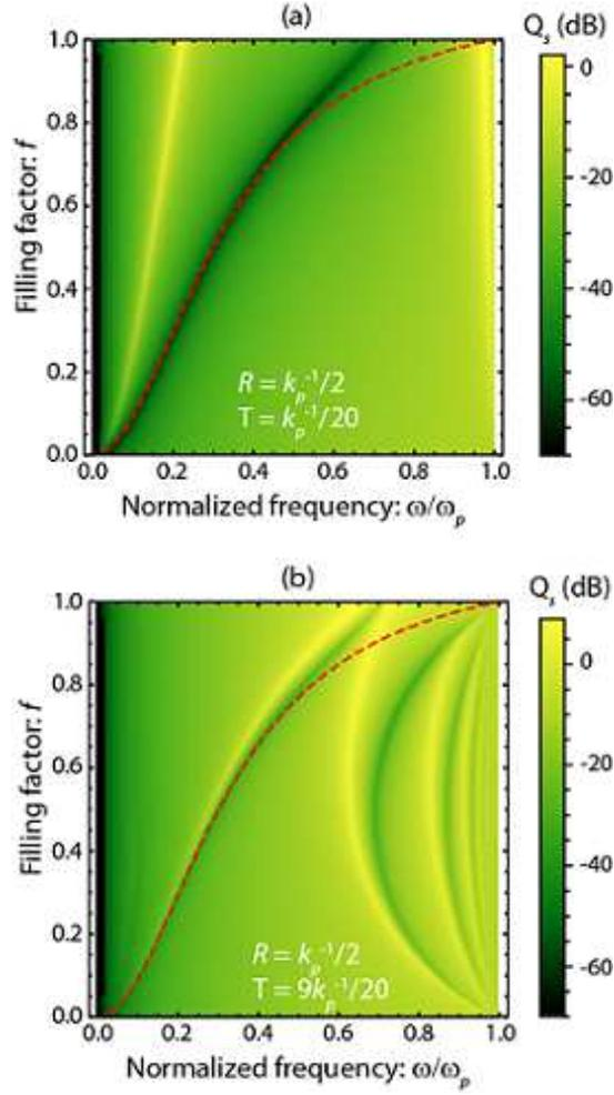
**Fig. 5** Scattering spectrum of a tubular cavity immersed in air ( $\epsilon = \epsilon_1 = 1$ ) with utmost radius  $R = k_p^{-1}/2$ , when the thickness of the shell is (a)  $T = 0.1R$ , and (b)  $T = 0.9R$ . The red dashed line indicates the frequency  $\omega_{zero}$  given in Eq. (18).
