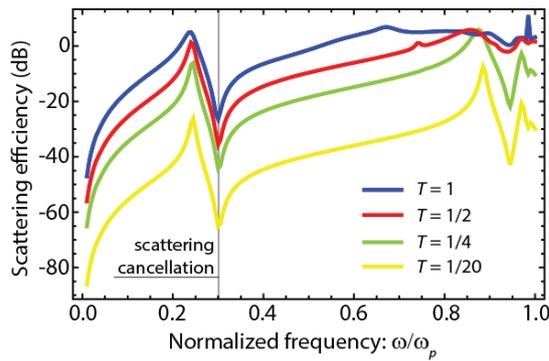
**Fig. 4** Scattering efficiency of metamaterial cavities immersed in air, where the aspect ratio  $T/R = 1/2$  is conserved. The tube thickness  $T$  is expressed in units of  $k_p^{-1}$ . The anisotropic metamaterial is again characterized by a filling factor of the Drude medium set as  $f = 1/2$ , where the damping rate is  $\gamma = \omega_p/100$ .
