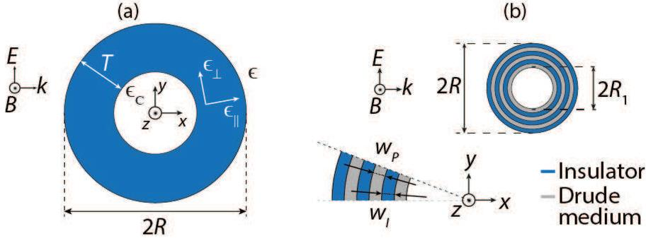
**Fig. 1** (a) Illustration of the anisotropic infinitely-long cavity. (b) Coaxial multilayered metamaterial establishing a radial-form birefringence.
