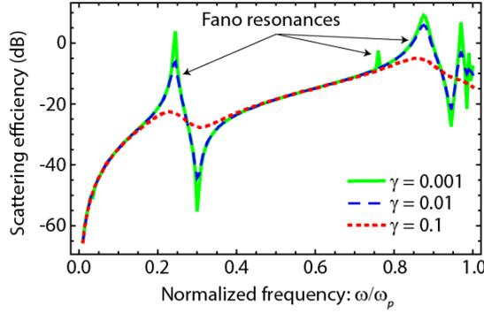
**Fig. 6** Scattering efficiency of a tubular anisotropic metamaterial ( $f = 1/2$ ) of equal radius and thickness,  $R = T = k_p^{-1}/4$ , immersed in air. The damping rate of the Drude medium varies from  $\gamma = 1/10$ , expressed in units of  $\omega_p$ , and  $\gamma = 1/1000$ .
