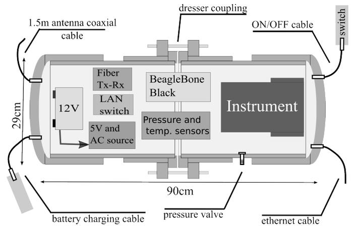
Fig. 6. Pressure vessel with approximated location of electronics.
