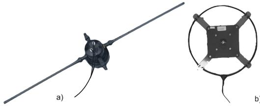
Fig. 7. Used antennas. (a) Dipole (insulated configuration). (b) 10-turns Loop.
