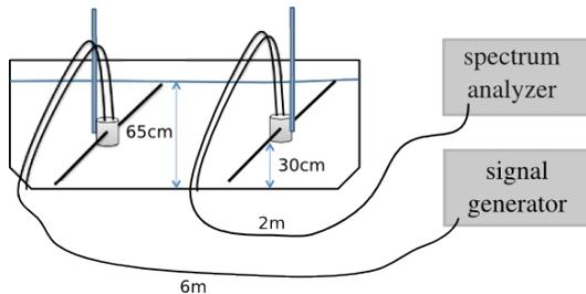
Fig. 2. Controlled indoors experiment.
