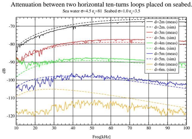
Fig. 9. Measurements vs. simulations. Low frequency sweep.
