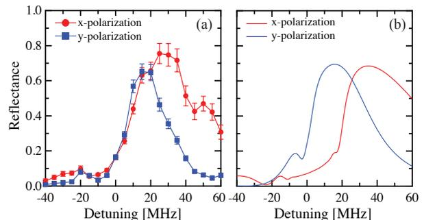
FIG. 5. (color online). Effect of the chiral character of the waveguide on Bragg reflection. (a) Measured reflection spectra for  $x$ - and  $y$ -quasilinear polarization, with  $\Delta\lambda = 0.2$  nm. (b) Theoretical simulations ( $N = 2000$ ,  $\Gamma_{1D}/\Gamma_0 = 0.007$ ,  $\Gamma_{1D}^{\text{forw}} = 2.8\Gamma_{1D}$ ,  $\Gamma_{1D}^{\text{forw}}/\Gamma_{1D}^{\text{back}} = 12$ ,  $f = 0.3$ ).
