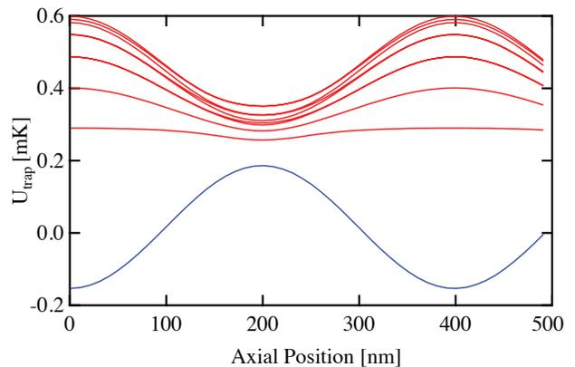
FIG. 9. Adiabatic trapping potential  $U_{trap}(z)$  for the near resonant trap for Cs atoms outside a cylindrical waveguide of 200 nm radius. Here,  $\Delta\lambda = 0.2$  nm and the red-detuned trapping power is  $2 \times 1.9 \mu\text{W}$ . The power of each blue-detuned fields at 686.1 nm and 686.5 nm is 4 mW. Blue line corresponds to the axial potential for the ground state manifold  $6S_{1/2} F = 4$ , while the red lines correspond to the substates of the excited state  $6P_{3/2} F' = 5$ .
