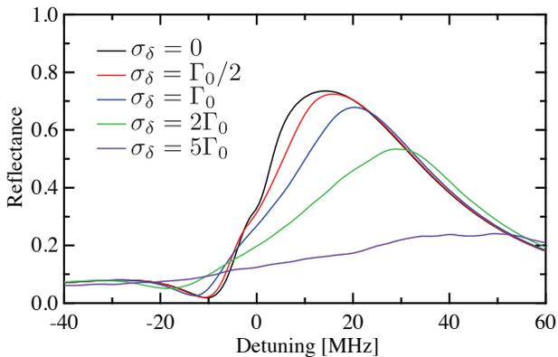
FIG. 7. Simulated reflection spectra for a probe quasilinearly polarized along the  $y$ -direction (symmetric decay rates) and different inhomogeneous broadening  $\sigma_\delta$ . The trap detuning is  $\Delta\lambda = 0.2$  nm, the number of atoms  $N = 2000$  and the decay rate  $\Gamma_{1D}/\Gamma_0 = 0.007$ . The spectra are averaged over 15 realizations.
