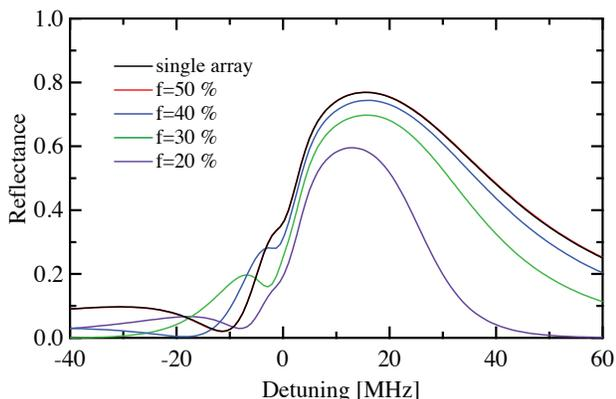
FIG. 8. Simulated reflection spectra for a probe quasilinearly polarized along the  $y$ -direction (symmetric decay rates) and a given filling factor  $f$  of each trapping site. We consider two parallel arrays. The trap detuning is  $\Delta\lambda = 0.2$  nm, the number of atoms  $N = 2000$  and the decay rate  $\Gamma_{1D}/\Gamma_0 = 0.007$ . The spectra are averaged over 15 realizations.
