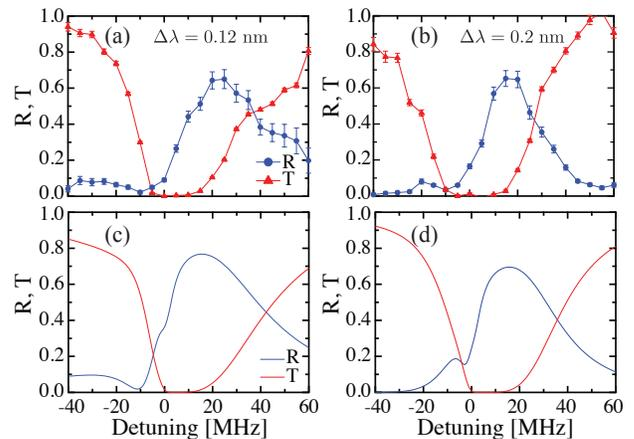
FIG. 3. (color online). Reflection and transmission spectra for a probe quasilinearly polarized along the  $y$ -direction. (a) and (b) Experimental results for  $\Delta\lambda = 0.12 \text{ nm}$  and  $\Delta\lambda = 0.2 \text{ nm}$ . (c) and (d) Simulated spectra for  $N = 2000$  atoms,  $\Gamma_{1D}/\Gamma_0 = 0.007$  and a filling factor of the lattice sites  $f = 0.3$ . The coupling value and filling factor have been adjusted to fit the measured spectra reported in (a).
