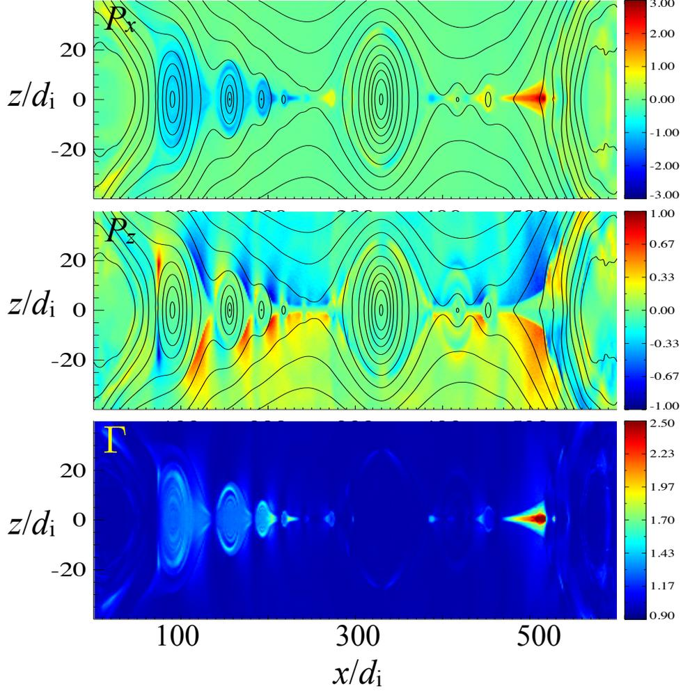
FIG. 3: The relativistic flows in the reconnection layer with  $\sigma = 100$ . Top panel: the bulk momentum in the x-direction  $P_x = \Gamma v_x/c$ , Middle panel: the bulk momentum in the z-direction  $P_z = \Gamma v_z/c$ , Bottom panel: the bulk Lorentz factor  $\Gamma$ .
