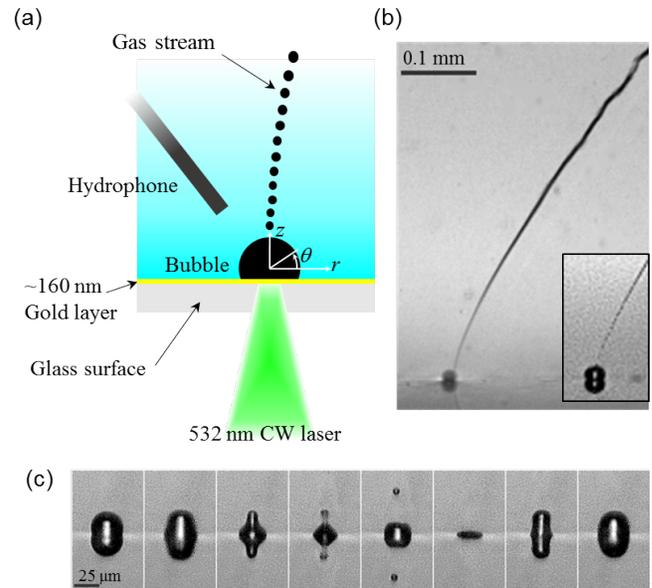
FIG. 1. Laser powered microheater: (a) A  $532\ \text{nm}$  CW laser ( $29.5\ \text{mW}$ ) is focused onto a thin layer of gold (around  $165\ \text{nm}$  thickness). (b) A bubble forms on the gold layer and sheds of microbubbles into the bulk (see inset). (c) Details of the bubble oscillation leading to the microbubble pinch-off at the bubble's apex.
