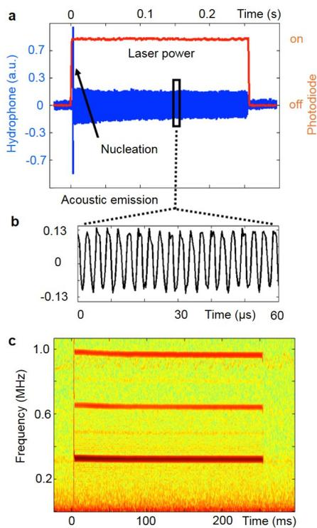
FIG. 2. Measurement of the bubble oscillation through acoustic emission. (a) The signal picked up by a hydrophone at nucleation and during continuous illumination with the laser beam. (b) Zoomed in region showing the sinusoidal signal oscillating with 320kHz. (c) The spectrogram depicts the fundamental frequency and higher harmonics at nearly constant frequency over the duration of the laser heating of 250ms.
