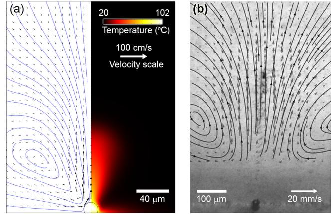
FIG. 4. a) Simulation of the heat transfer (right) and the thermocapillary induced flow (left) of a steady bubble under laser irradiation of  $40\text{ mW}$ . b) Flow field obtained from particle image velocimetry with  $2\mu\text{m}$  diameter particles. Due to illumination constrains we could not identify particles in the bottom part of the image. Note the different image scales on the left and right figure.
