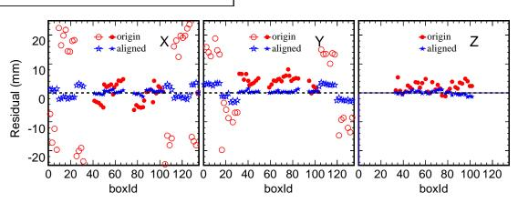
Fig. 2. Residuals in x-, y-, z- directions. The dashed line is the reference at zero, red circles and dots are before alignment, blue stars are after alignment. The barrel is aligned by cosmic ray events (solid markers), the endcaps (hollow markers) are aligned by di-muon events.
