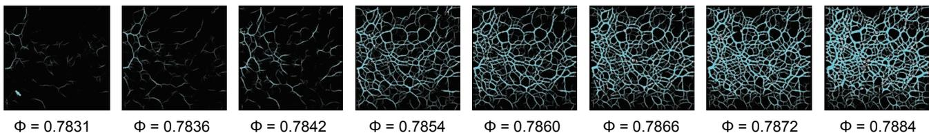
FIG. 2. **Evolution of the force network.** Photoelastic images of the system, taken at a sequence of eight steps above  $\Phi_J \approx 0.7825$ . The corresponding network of (normal) forces is overlaid on top of each picture. The collection of these static networks may together be represented as a single multilayer network that captures the evolution of the granular system throughout compression.
